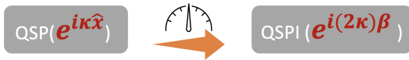
Figure 4.4: Pictorial illustration of how in the bosonic QSP interferometric protocol, the qubit measurement enacts a duality between a polynomial transformation on the bosonic quadrature operators and a polynomial transformation on the sensing parameter \beta via QSPI.
