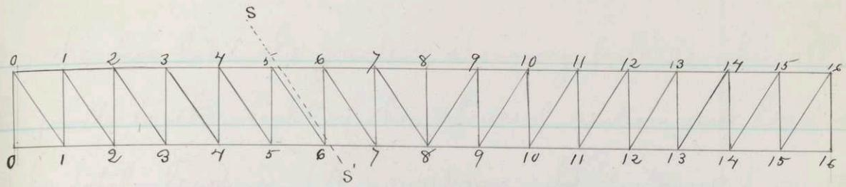
the of divisions in the truss. The posts and diagonals are numbered by the number of the joint where their lower ends meet. The divisions of the upper chord are numbered by the greater number of the joints it lies between, those of the lower by the less. Let  $k$  denote the height of the girder measured from centre to centre of the pins in the upper and lower chords;  $s$ , the length
