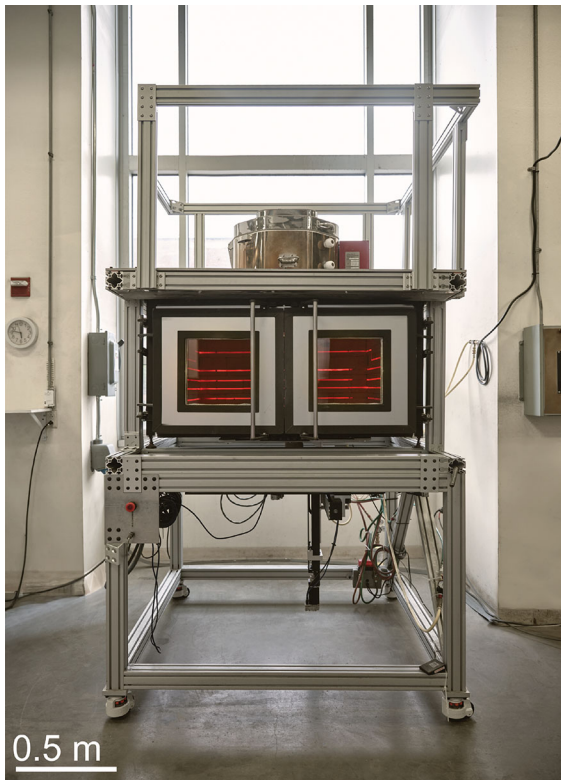
Fig. 1 G3DP3 shown in its current configuration. The build chamber is shown behind the glass pane doors. Above it are the furnace kiln and crucible
