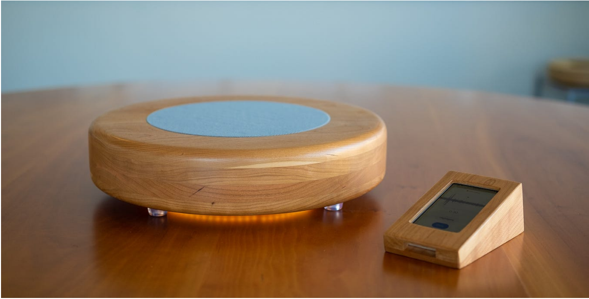
Figure 2-1: Photo of version 2 of the Hearth by Cortico. The Hearth is the recording device used to collect the in-person accounts of those who participate in a Fora small group, facilitated dialogue.
