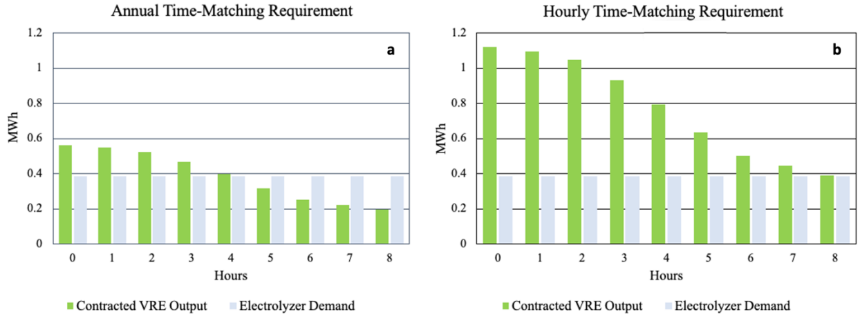
Figure 1: Simplified illustration of annual vs. hourly time matching. Electricity demand and contracted VRE resource output under an annual (a) and hourly (b) time-matching requirement simplified such that the requirements are only enforced over eight hours. In the annual plot, aggregate electrolyzer demand is equal to aggregate output from the contracted VRE over the eight hours, which corresponds with over generation in some hours and under generation in other hours. In the hourly plot, contracted VRE output is greater than or equal to electrolyzer demand in each hour. To accomplish this, the VRE resources has to be sized at a higher capacity. Both subplots use the same VRE generation profile, but the capacity is sized to the minimum required to meet the relevant requirement. In practice, to meet the H 2 PTC hourly requirement a mix of VRE, batteries, and H 2 storage with flexible electrolyzer operation can be deployed.
