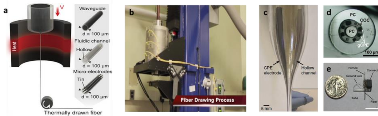
Figure 1.7. (a) Schematic illustration of the thermal drawing process that shows a preform that is predominantly composed of thermoplastic polymers being heated in 3-zone furnace and drawn into several kilometers long fibers with microscale features that remain conserved in the entire length, figure reproduced from Ref. 28 28 ; (b) Photograph of the thermal drawing tower that I used for all of my draws; (c) Pictures showing the necking-zone of an all-polymer preform, figure reproduced from Ref.26 26 ; (d) Cross-sectional micrograph showing the embedded features in the corresponding fiber that results from this preform, figure reproduced from Ref.26 26 ; (e) Fully assembled device, figure reproduced from Ref.26 26 .
