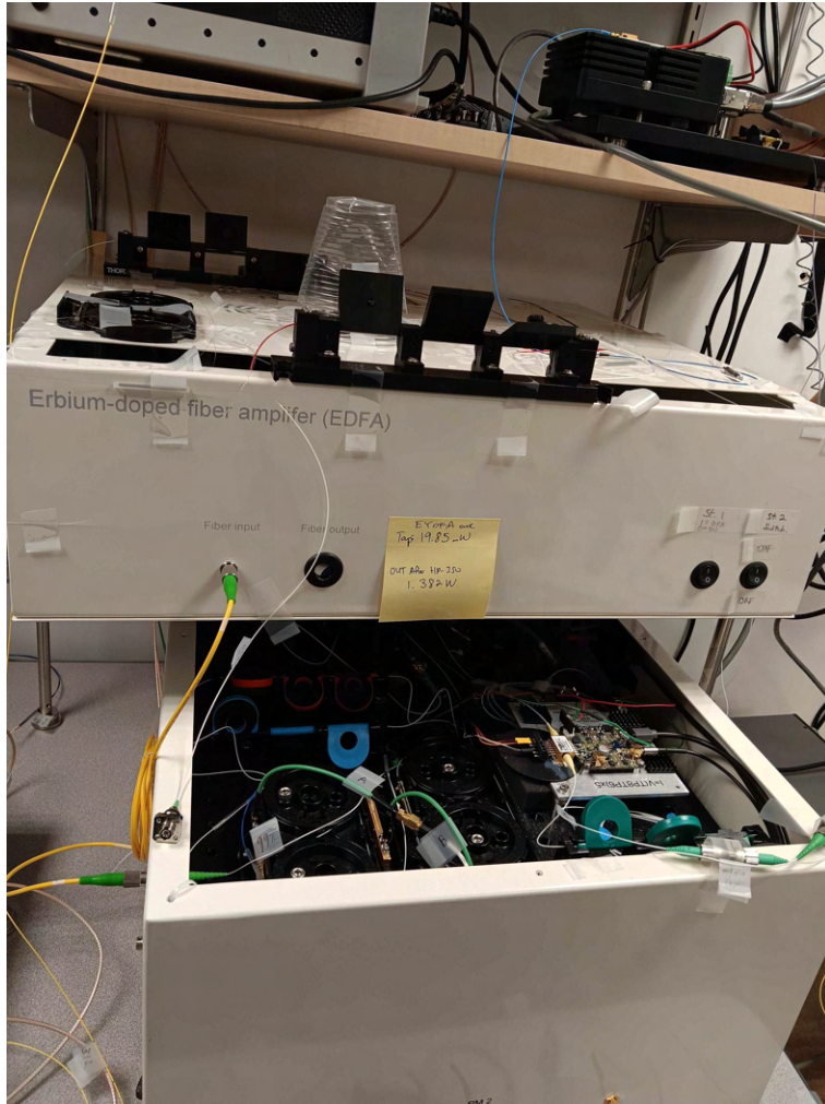
Figure 3.7: Packed EYDFA module. The output fiber was temporarily taken out for testing. The module was placed right on top of the time-stepped frequency comb source box on the bottom.
