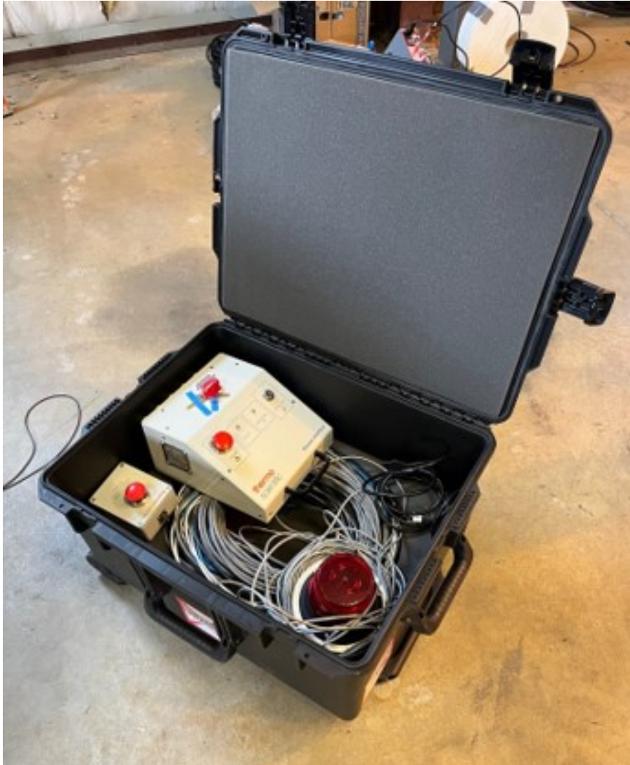
Figure B-8: Photograph of the D-T Generator equipment and cables inside a wheeled protective case. Foam packing has been removed for visibility. There is sufficient room for the D-T tube itself, however this was transported in a separate wheeled case by EHS personnel during field experiments.
