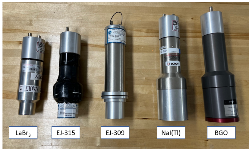
Figure 3-8: A photo of the five detectors selected for this study, specifications available in Table 3.2
