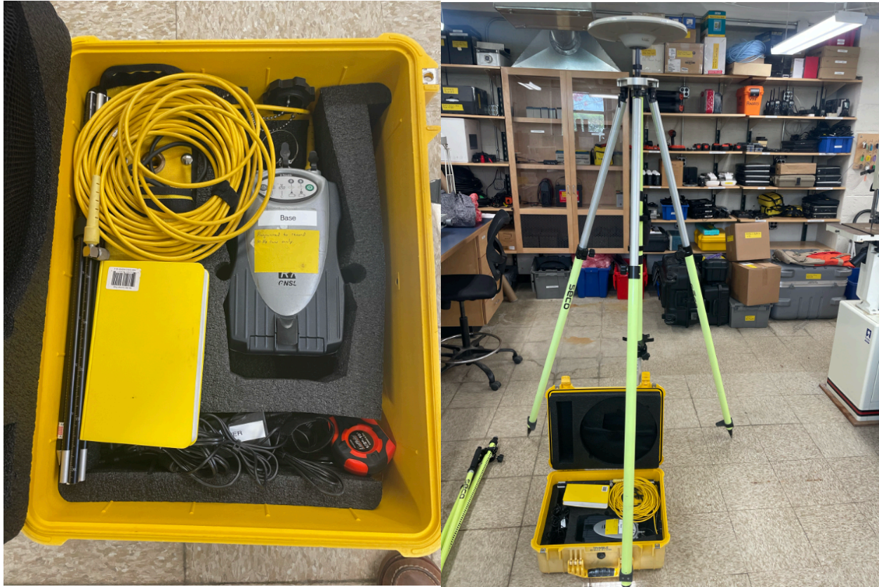
Figure 3.1: Backpack apparatus with Trimble GPS receiver in yellow box on the left and the base station tripod and accompanying Trimble GPS antenna on the right.
