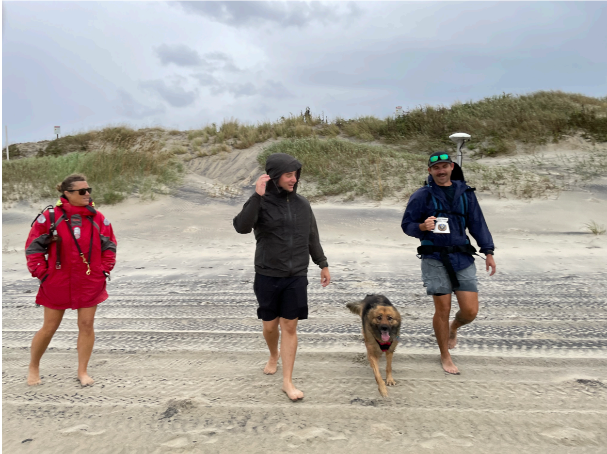
Figure 2.2: Daily backpack surveys between the dune toe and the ocean were conducted requiring walking ~5-6 km (~100-120 km over the 3-week study). The backpack contains a strap and harness system housing a Trimble R7 GPS receiver with an attached Trimble Zephyr Geodetic antenna.
