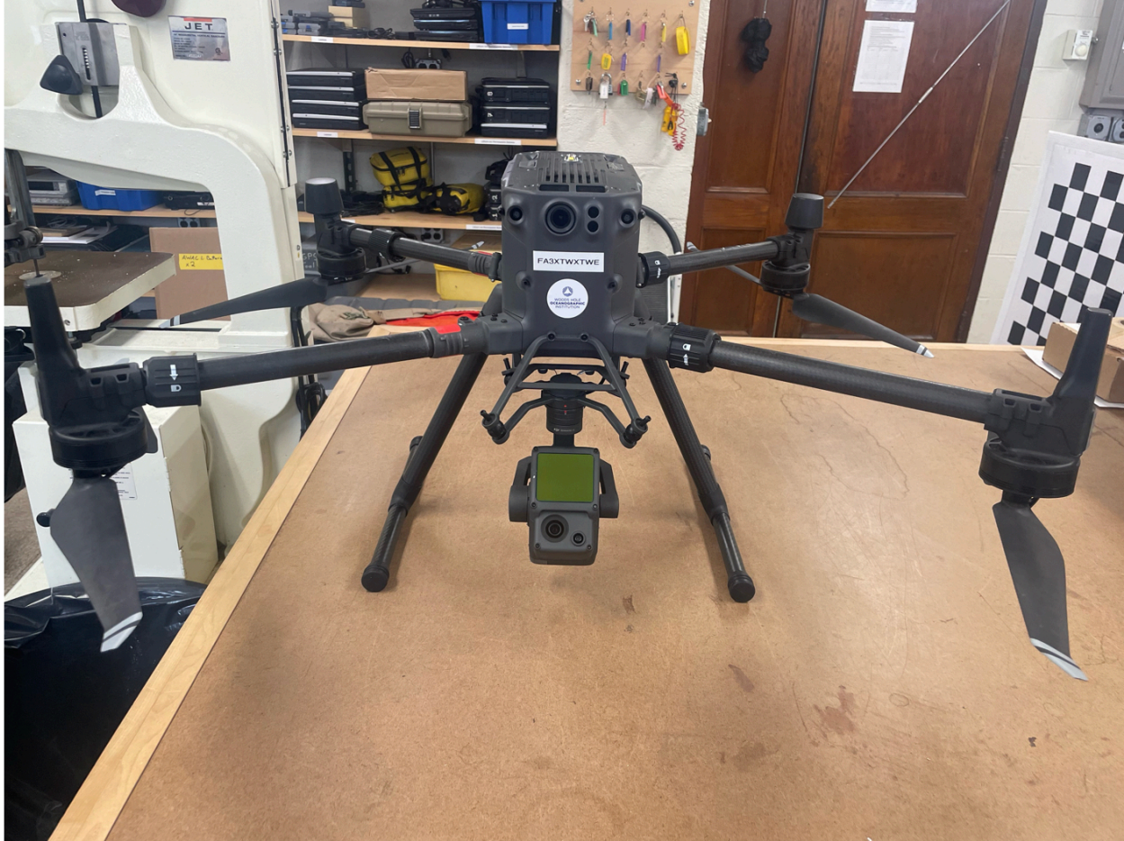
Figure 3.2: DJI Matrice M300 with Zenmuse L1 payload attachment.
