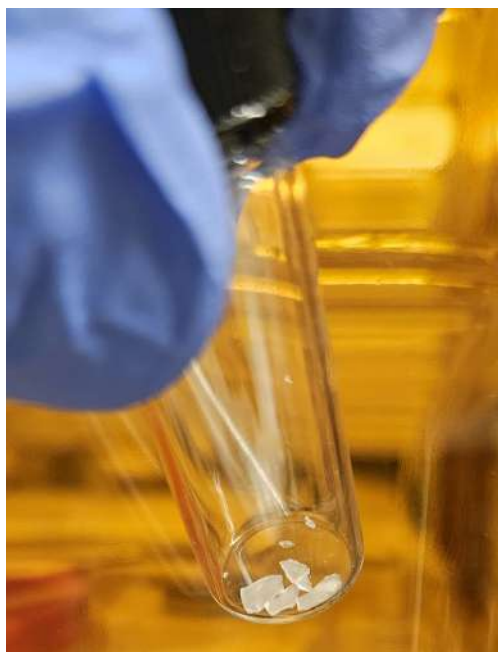
Figure 5.4: EPR samples : fragments of Exail IXF-RAD-SM-1550-014-PI fiber preform in a glass jar.
