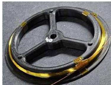
Figure 2.4: Original optical fiber plastic spool (Spooling diameter: 9 cm)
