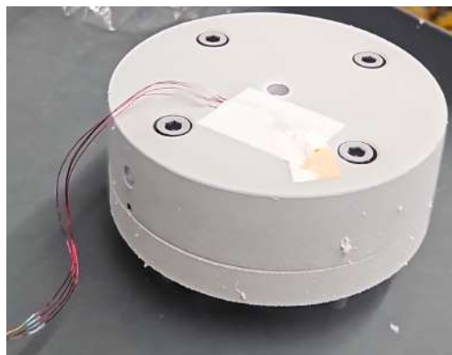
Figure 2.7: Picture of the spool during ambient temperature warm-up test after liquid nitrogen cool-down
