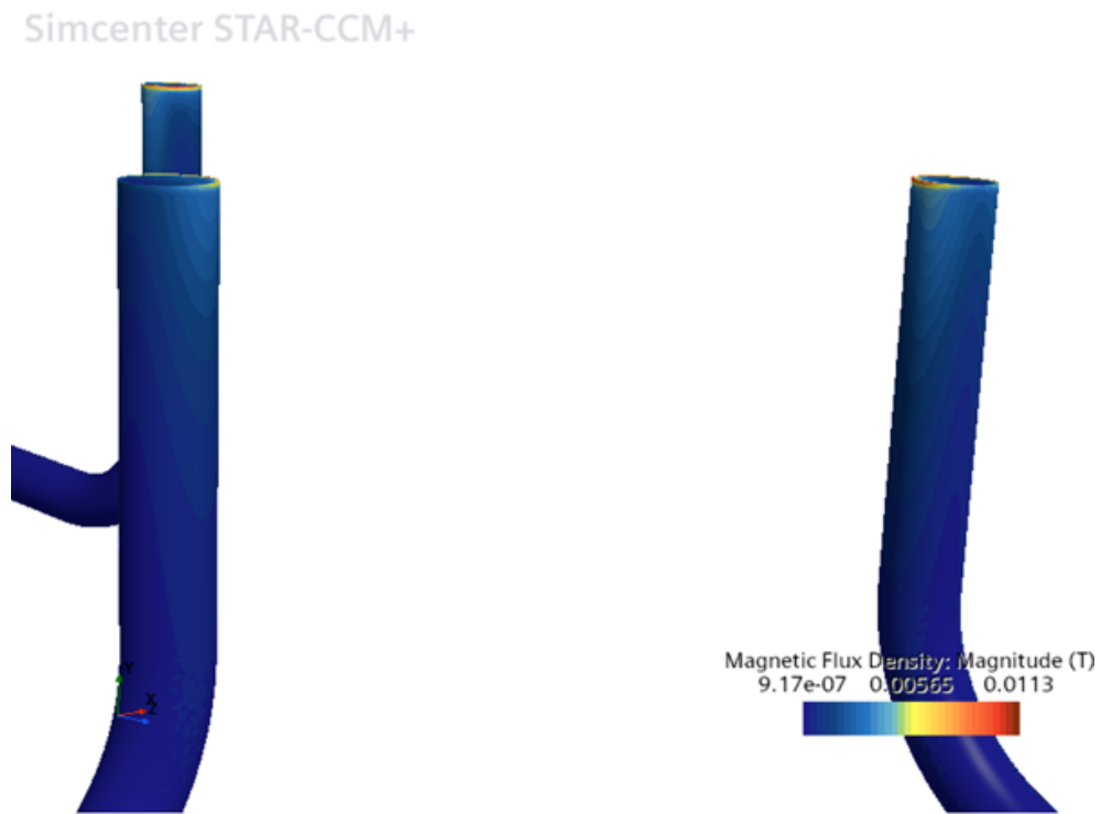
Figure 5.19: Magnetic flux at peak time step for 430 kHz operations of Heat Pipe iteration 3.
