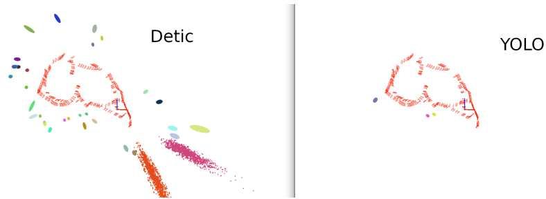
Figure 3.7: Semantic map of objects and trajectory of YOLO and Detic GAPSLAM produced in the Vicon 3 dataset for an object detection score of 0.65. Object classes are not labeled in the figure, but is recorded and can be retrieved.
