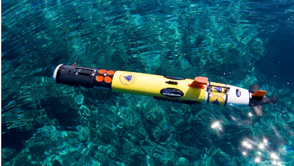
Figure 1.3: Image of a REMUS 100 unit created by WHOI and Kongsberg Maritime. During Operation Iraqi Freedom in 2003, the U.S. Navy used REMUS vehicles to detect mines in the Persian Gulf harbor. Navy officers said they preferred REMUS AUVs because each could do the work of 12 to 16 human divers, and they were “undeterred by cold temperatures, murky water, sharks, or hunger.” [21]
