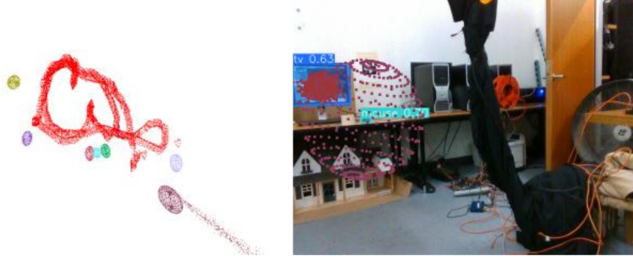
Figure 2.4: GAPS LAM image showing relation between the current update of the map being generated to the current video frame processed by front-end. The purple Gaussian appears as an ellipsoid on the map and sphere in the video, while the orange particle filter has a cone shape on the map while having a more rounded appearance in the video. The difference comes from the map being presented from a bird’s-eye view downwards perspective while the video is recorded from a human-eye level forward facing perspective.
