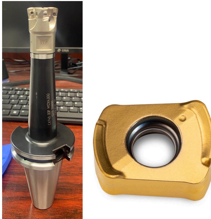
Figure 10: Image of Ingersoll 1TG1V-10013X7R01 tool assembly (left) and insert (right) [9]
