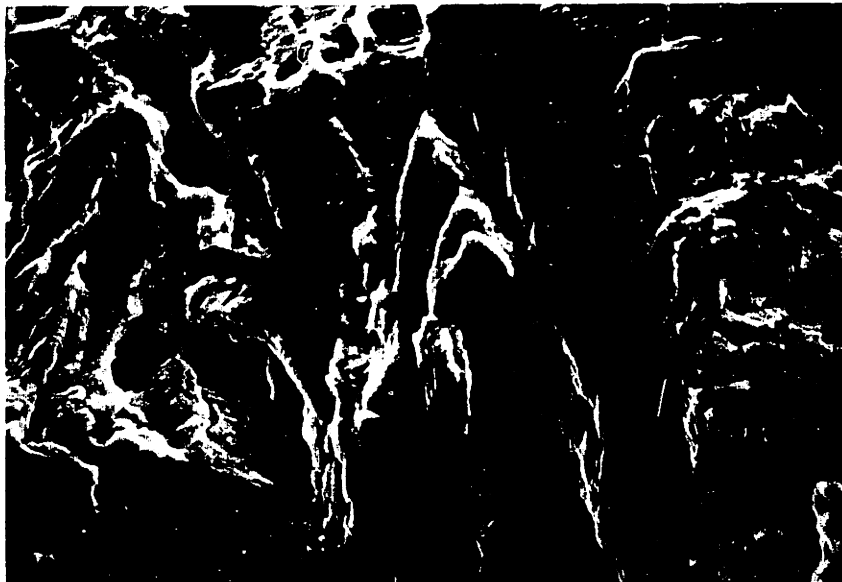
Figure 7.34 Fracture Surface of Desensitized Alloy-600 Showing Crystallographic Crack Path With Striations, 2000X. Crack Path from Bottom to Top. \Delta K Approximately 20 MPa \sqrt{m} .
