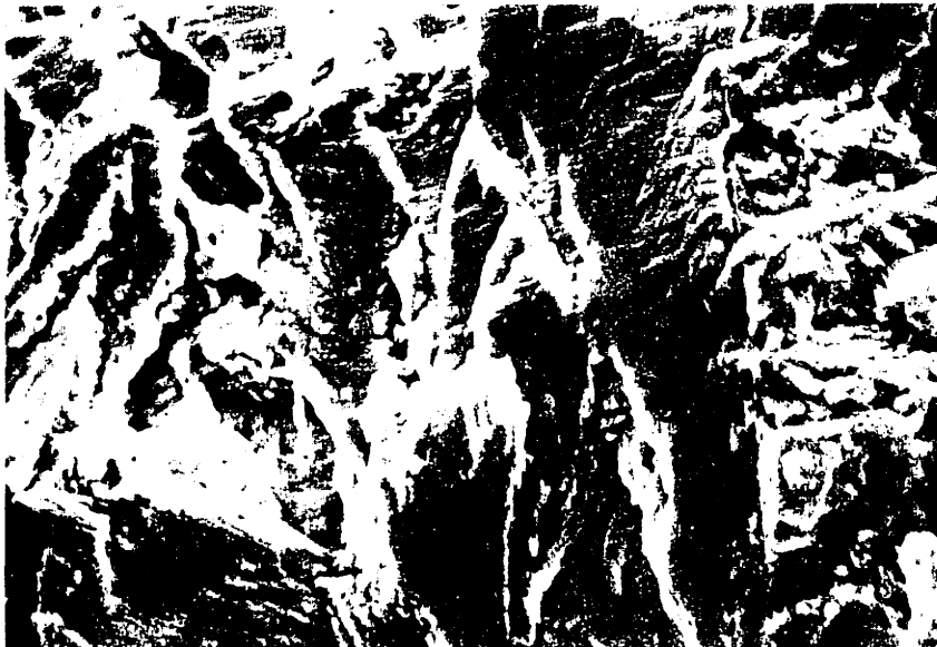
Figure 7.34 Fracture Surface of Desensitized Alloy-600 Showing Crystallographic Crack Path With Striations, 2000X. Crack Path from Bottom to Top. K_{IC} Approximately 20 MPa \sqrt{m} .
