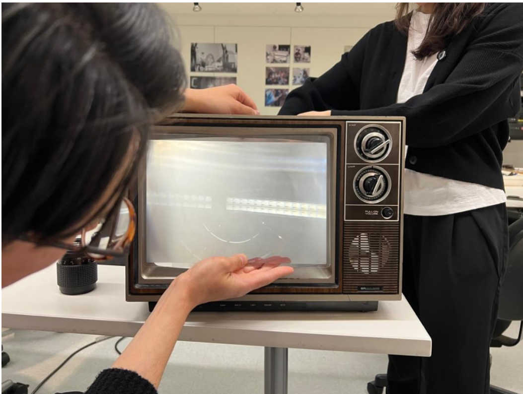
Figure 5.6. Prototyping the combination of TV case, Fresnel lens, and diffuser panel that would be used to make the work.
