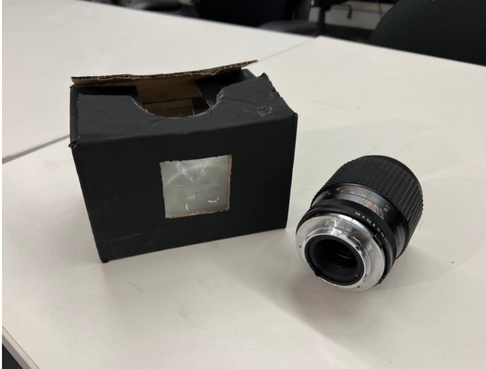
Figure 5.7. Prototyping the combination of hard-stock paper box, film camera's focusing screen, and mirror.
