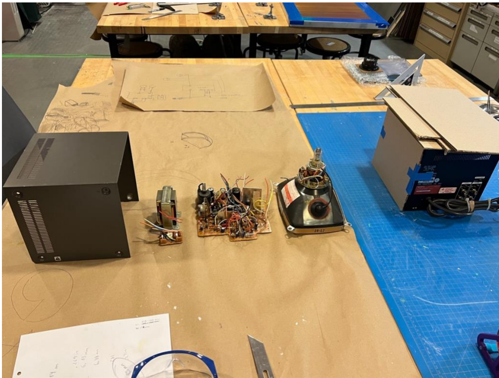
Figure 5.8. Work in progress documentation of disassembling the CRT TV.
