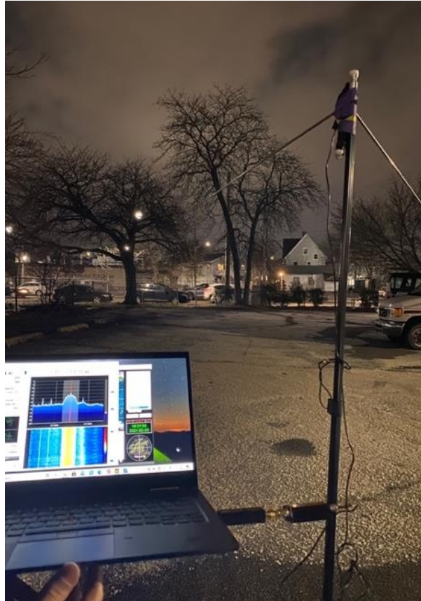
Figure 1.1. Documentation of my antenna setup: dipole antennas connected to an RTL-SDR device, which is linked to my laptop to receive signals from weather satellites.
