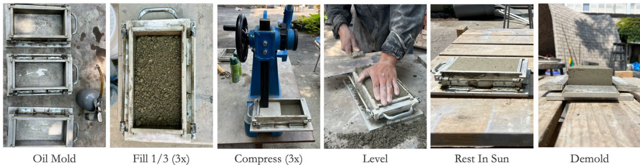
Figure 23: summarized procedure for brick compaction
