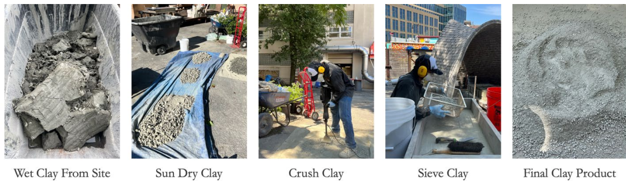
Figure 20: Procedure to prepare Boston blue clay for mixing.
