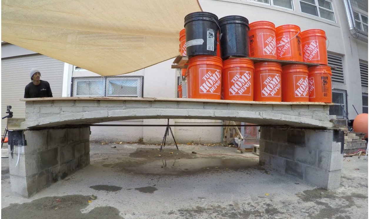
Figure 43: Fifty buckets full of water on half of vault during 4 kN/m 2 asymmetrical loading
