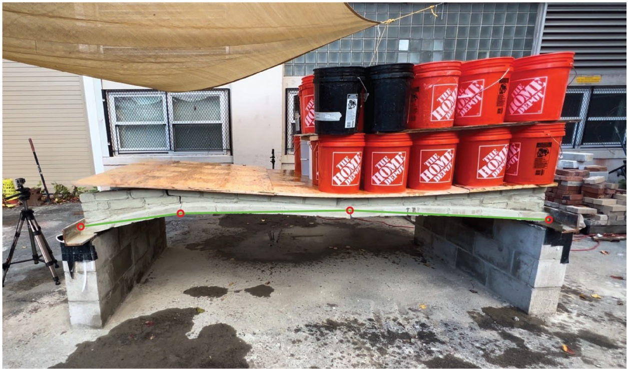
Figure 44: Vault at moment of collapse showcasing three bar hinge mechanism
