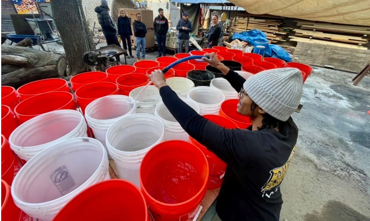
Figure 41: Twenty-five buckets being filled with water during 2 kN/m 2 asymmetrical loading
