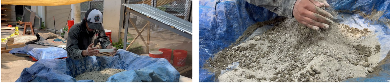
Figure 21: Incremental moistening of soil mixture
