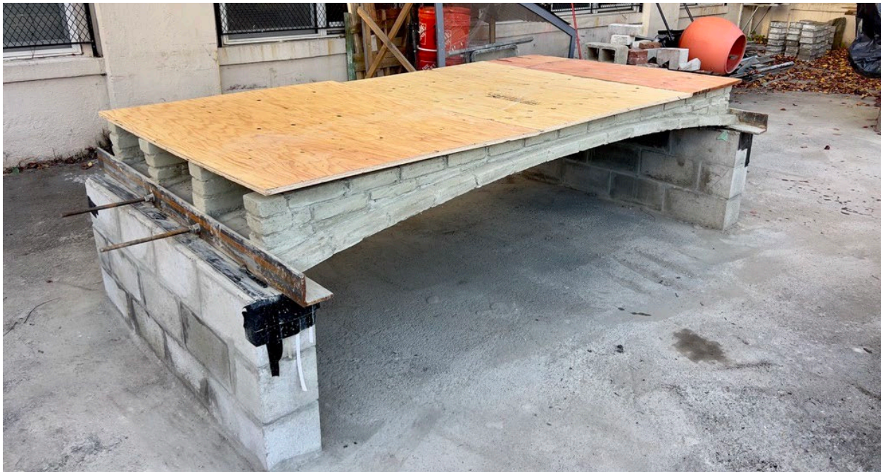
Figure 38: Completed vault floor prototype perspective view
