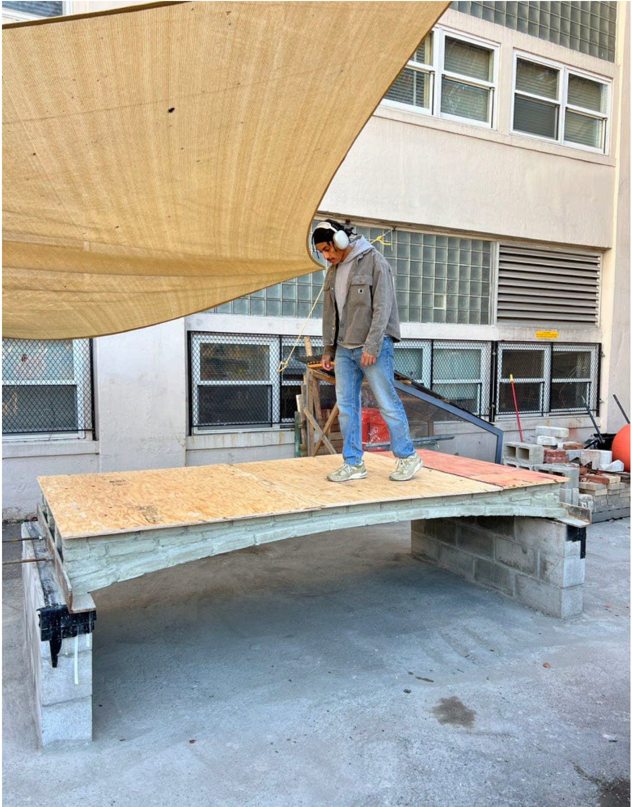
Figure 40: Completed vaulted floor prototype with author walking on top
