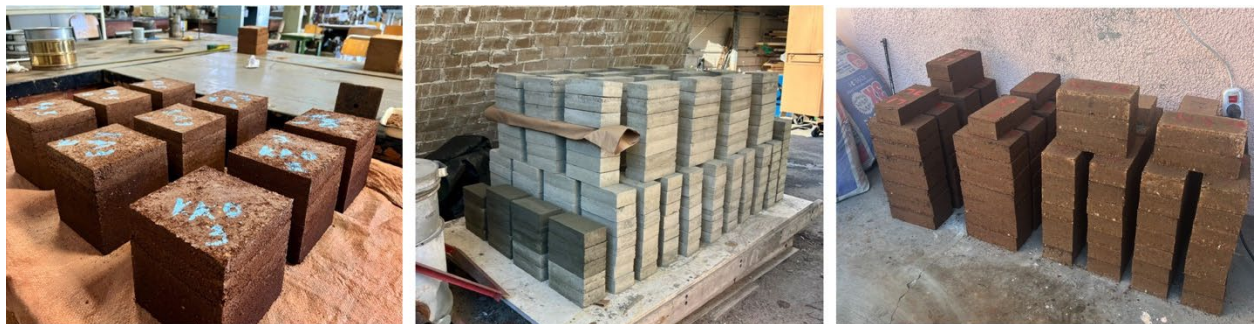
Figure 14: Various compressed stabilized earth bricks in Addis Ababa, Ethiopia and Boston, Massachusetts
