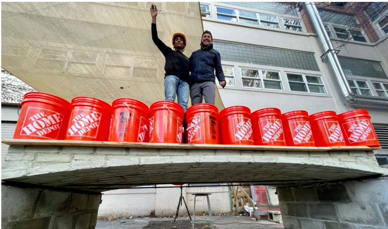
Figure 42: 2 kN/m 2 symmetric load case with 1.25 kN point load at center
