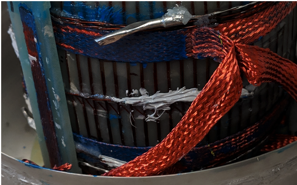
Figure 4-2: Close-up image of the ABRA magnet wires, the wire only appears to cross in one direction as the wire is wound between Delrin wedges and does not cross back, suggesting that the magnet was not counter-wound.
