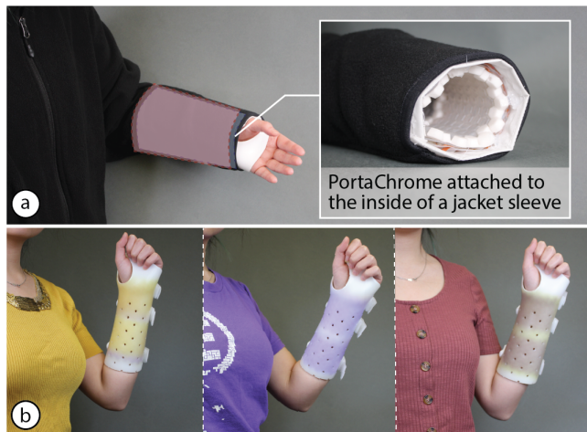
Figure 16: (a) PortaChrome can be attached to the inside of the sleeves to (b) reprogram the user’s wrist splint so that it matches the user’s daily outfit.
