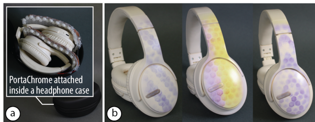
Figure 17: (a) Reprogramming headphone appearances by integrating PortaChrome with the original headphone case. (b) Three headphone designs were achieved with PortaChrome.
