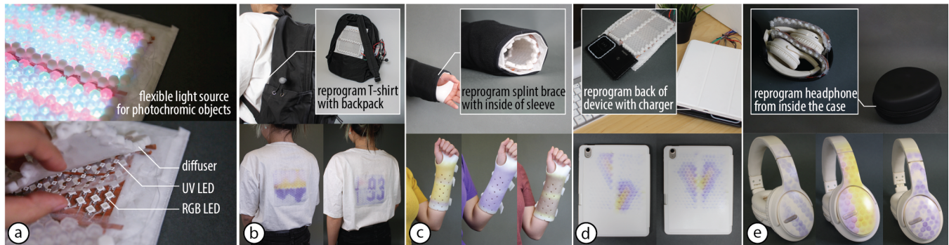
Figure 1: (a) PortaChrome is a flexible contact light source that can reprogram the appearance of an object previously coated with photochromic material. PortaChrome has integrated UV and RGB LEDs that saturate and desaturate the color channels of photochromic material. PortaChrome is portable and flexible, allowing it to be attached to (b) a backpack to reprogram the back of clothes, (c) the inside of a sleeve to reprogram a splint brace, (d) a wireless charger to reprogram the back of a device, and (e) the inside of a headphone case to reprogram the design of a headphone.
