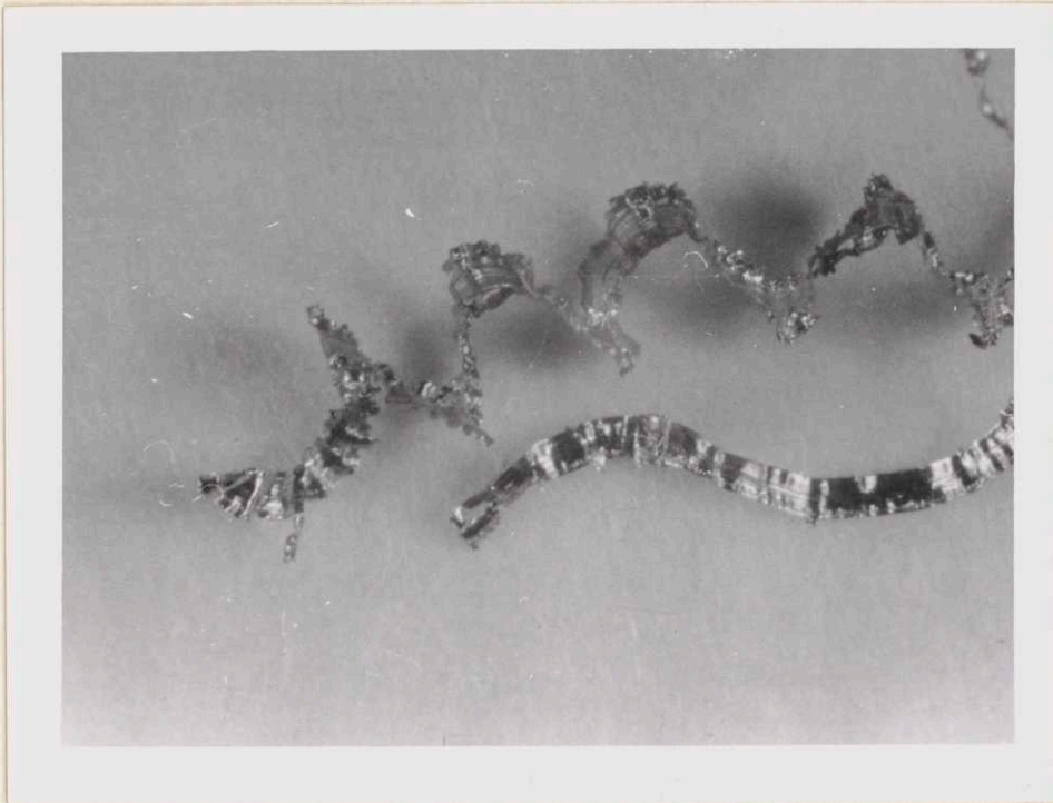
TITANIUM CHIPS SHOWING REWELDING (Upper chip is 1/4" in largest dimension)
