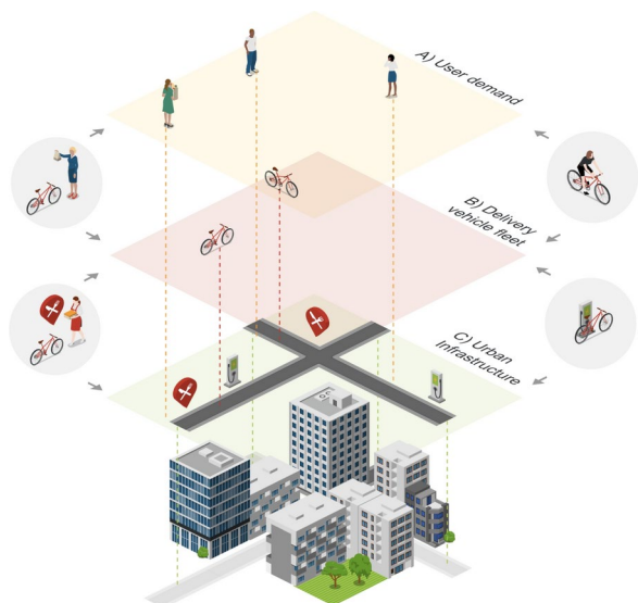
Fig. 1 Multilayer architecture of the model and interactions across layers: a urban infrastructure (buildings, roads, charging stations), b autonomous micromobility fleet which could include any single-person low-speed autonomous vehicles, and c user demand, including rides and food deliveries
