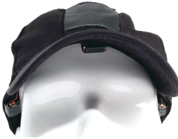
Figure 3-2: Prototype Bone Conduction Haptic Device
