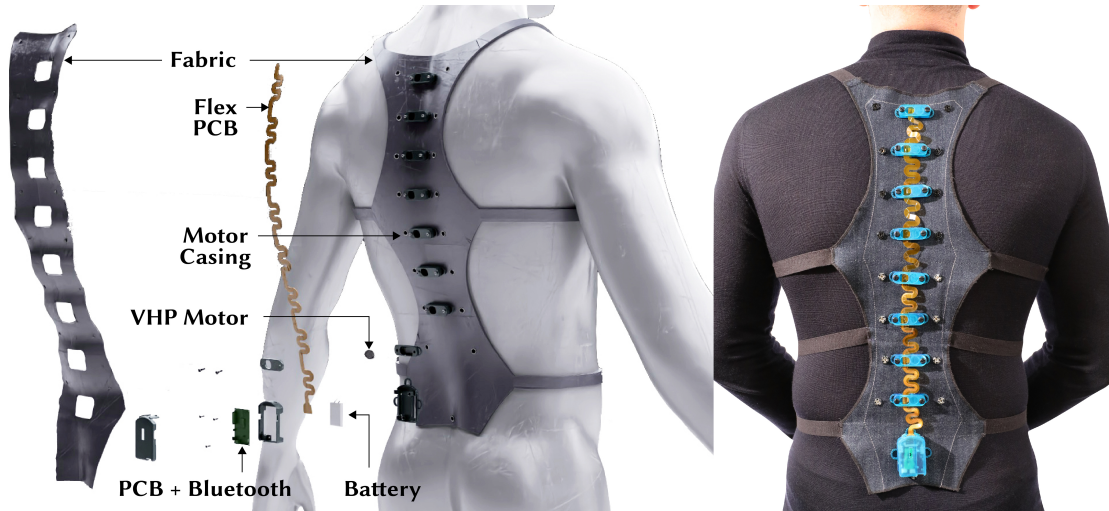
Figure 4-2: Overview of the haptic device. It is a vest like wearable with eight vibrotactile modules evenly distributed along the spine. The haptic device can be controlled by our web-based learning interface via Bluetooth.
