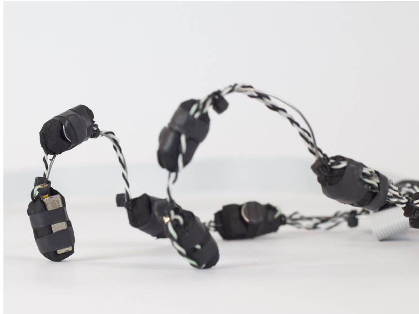
Figure 6-8: A closeup featuring both actuators. The circular one is the G1040003D, and the rectangular one is the VG0832022D.
