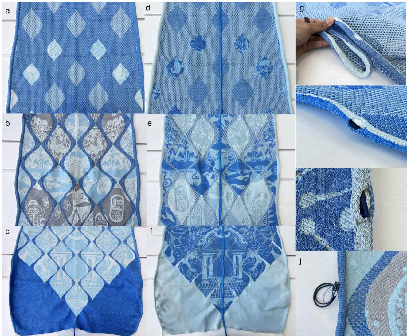
Figure 4.29: a-c) Front-side and d-f) back-side of a Living Knitwork panel. g-h) Channel openings that can be used to thread in electrical cabling and anchoring ropes. i) Multi-layer stranded wires are used to ground and shield every AC-transmission wire, protecting from external noise and pick-ups. Wires are crocheted to the knitted conductive textiles to ensure strong connection. j) First-stage transimpedance amplifier circuit beside the knitted receiver that can be slid into the channel.
