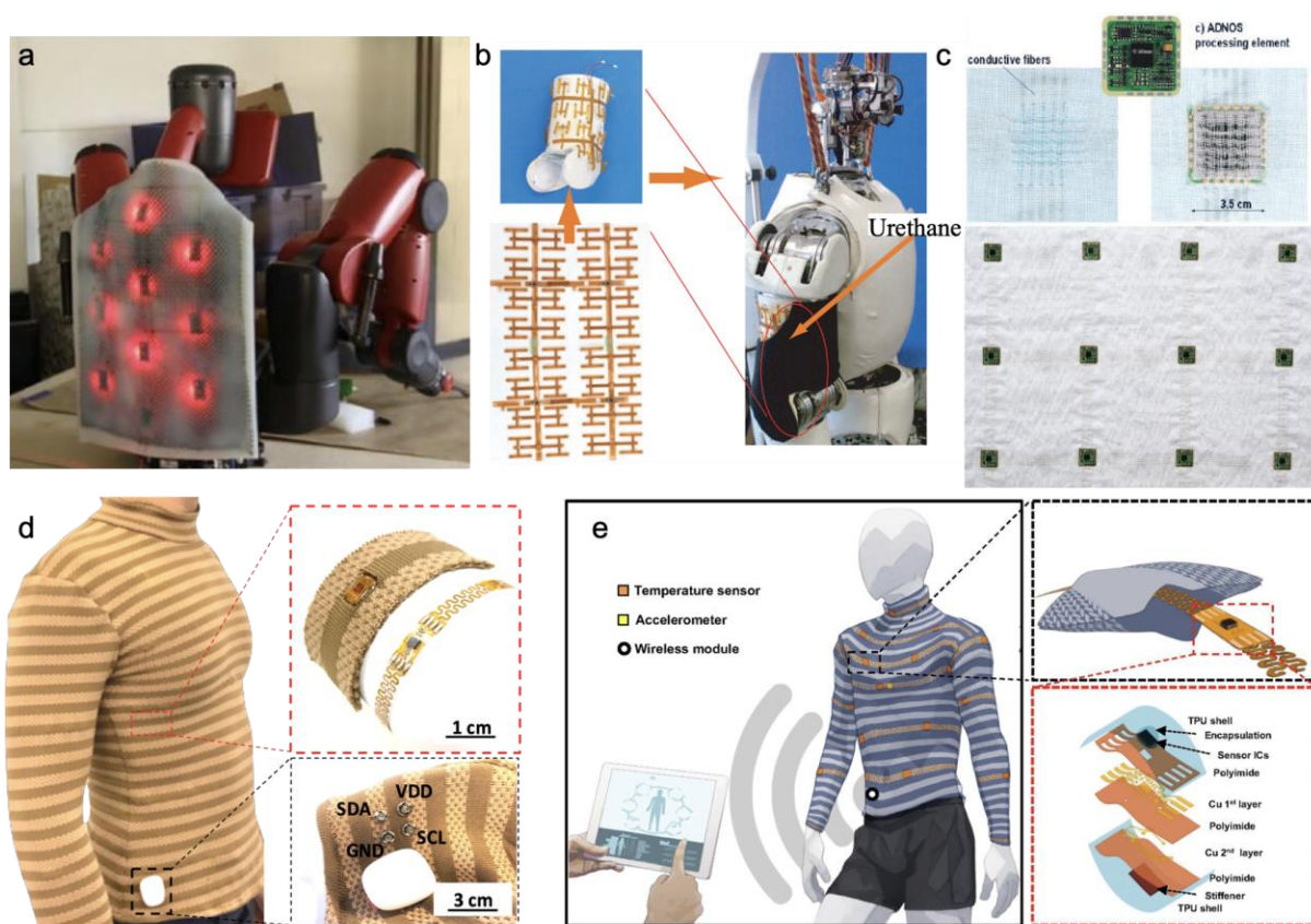
Figure 6.2: a) A soft, amorphous texture-sensitive skin from distributed microphones mounted on the back of a Baxter robot, b) Foldable tactile sensor network that can be embedded in deformable substrate for robotic skin, c) A large-area distributed embroidered capacitive sensing textile sensor, d-e) Electronic textile conformable suit (E-TeCS) with stretchable sensor network for large-scale spatiotemporal physiological sensing.
