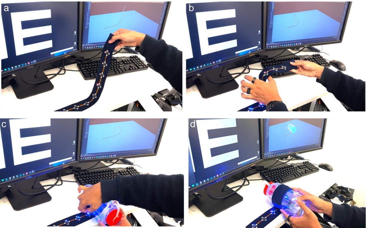
Figure 6.29: a-b) Shape-sensing and c-d) circumferential measurement based on 1D Network of NETS.
