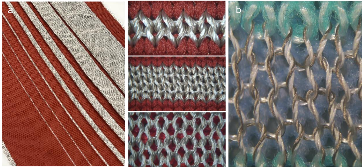
Figure 3.12: Samples of conductive textiles knitted with silver-plated yarns with multiple stitch rows (1,2,4,8,16, and 32 rows in wale direction) and their zoomed-in view a) with 2-ply of conductive yarn and b) with 1-ply of conductive yarn.
