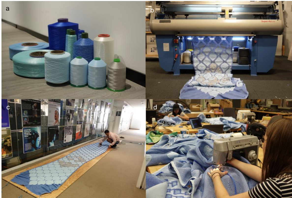
Figure 4.28: a) Various recycled polyester and functional yarns that make up five input spools used to fabricate the Living Knitwork petals. b) The knitting process. c) A custom large textile mold with wooden boards and nails were fabricated and used to stretch the panels. The textile panels are stretched by threading sailing ropes through both of the channels and securing them to designated nails before the thermoforming process. The low-melt yarns are activated through iron-steaming to fix the shape and size of all of the Knitwork petals. d) Dyneema ropes sewn with industrial sewing machines and heavy-duty yarns for central-line reinforcement.
