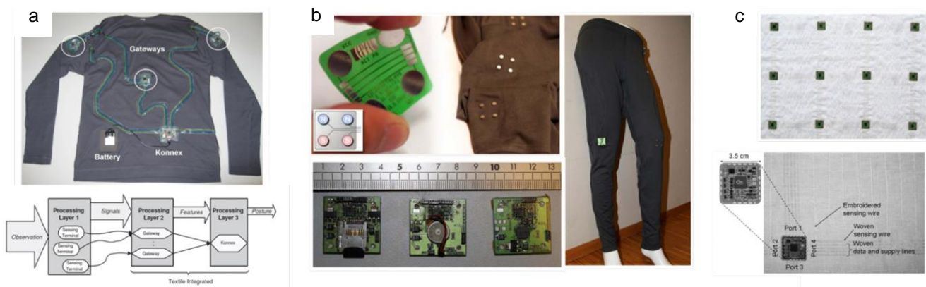
Figure 2.17: Distributed sensor network on textiles: a) multiple accelerometers connected to the main processing module through gateways for posture recognition garment [131], b) magnets as mechanical and electrical connectors to the bus for personalized wearables [132], and c) self-organizing and fault-tolerant distributed sensor network on fabrics based on capacitive conductive fibers [133].
