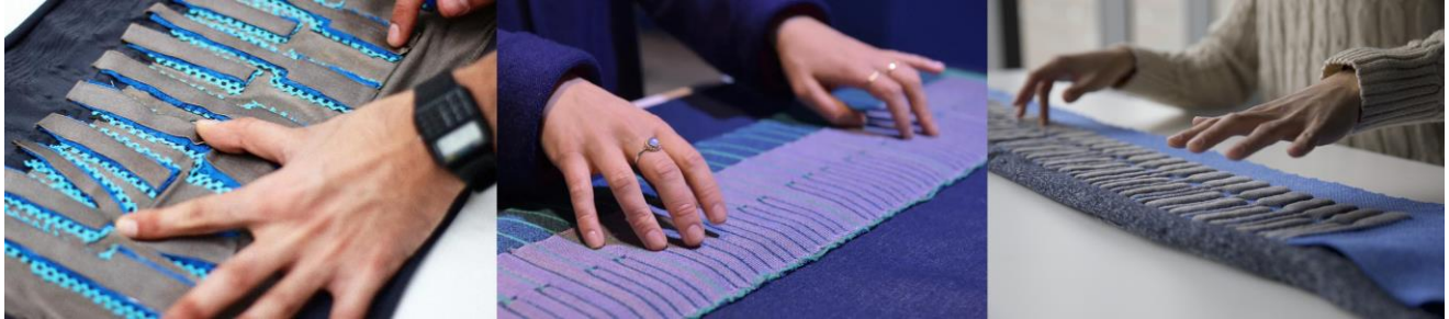
Figure 4.5: Evolution of prototypes from FabricKeyboard, KnittedKeyboard I, to KnittedKeyboard II
