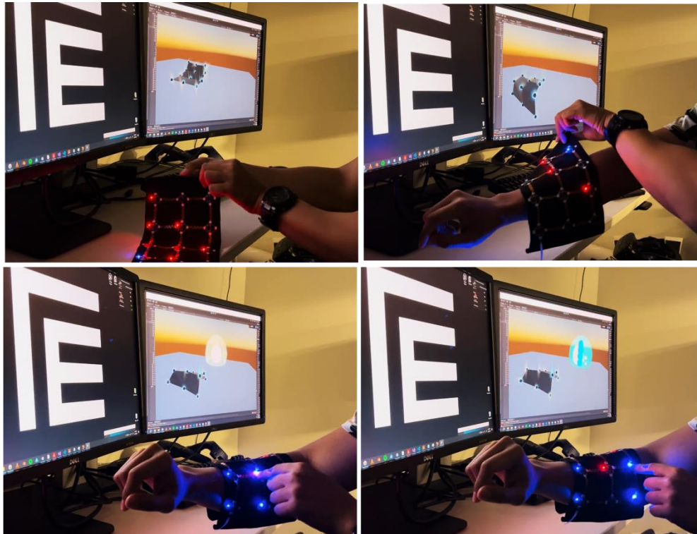
Figure 6.36: VR digital-twin of NETS with 12 nodes: a-b) the smart sleeve being wrapped onto an arm, c-d) the nodes can then be used as a controller.
