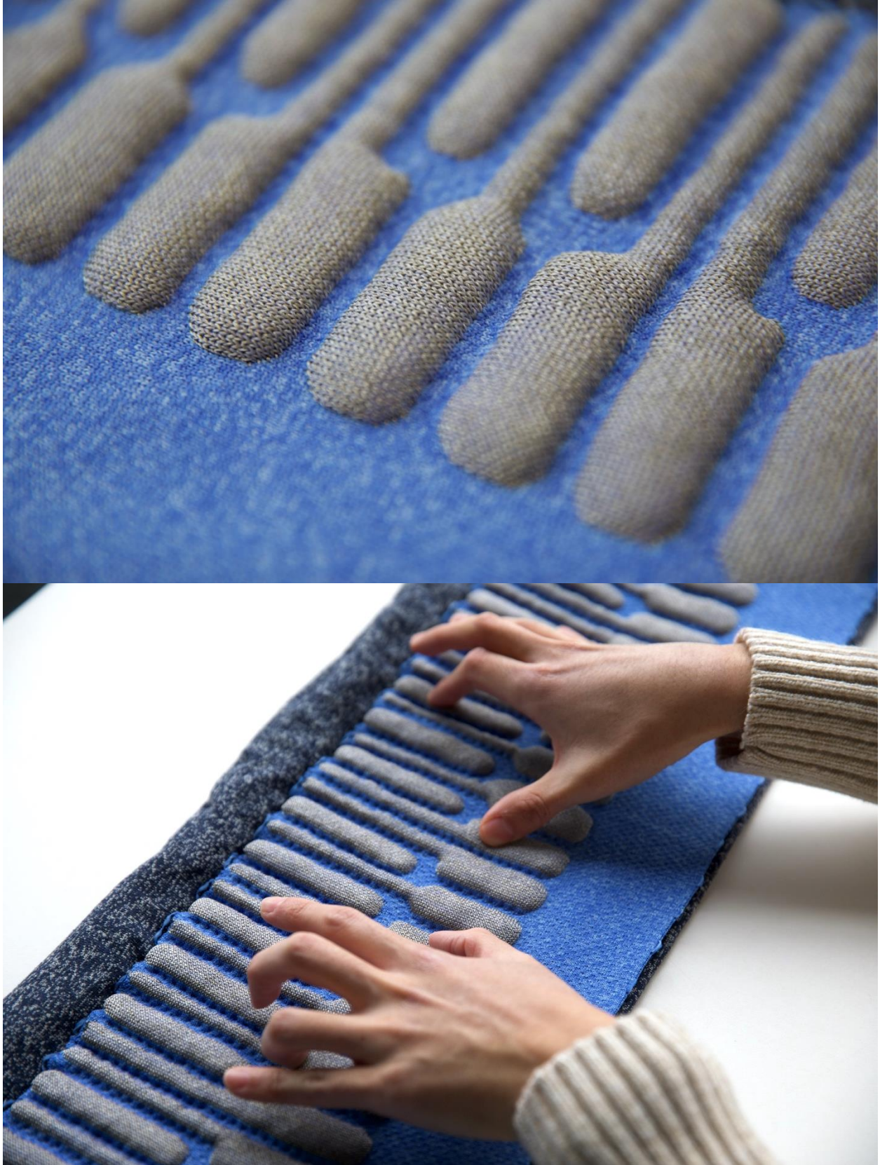
Figure A.1: Close-up images of KnittedKeyboard .
