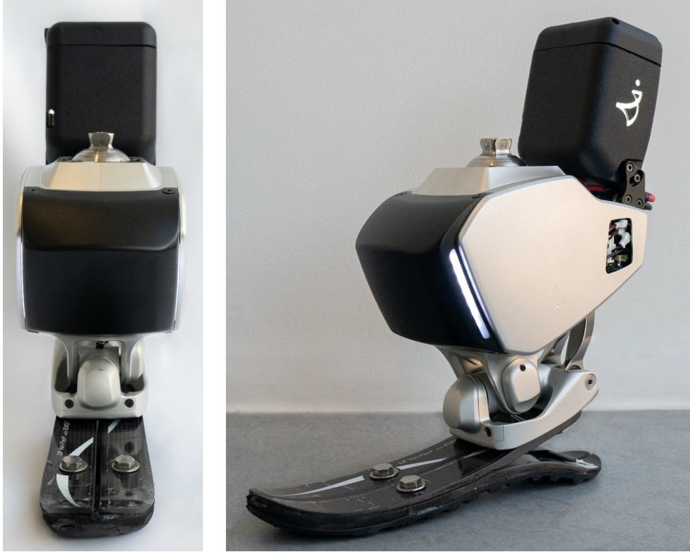
Figure 3-22: Front (left) and side (right) views of the developed prosthetic ankle device. The design incorporates a sleek, biomimetic form factor with integrated electronic components, showcasing the fusion of advanced robotics and ergonomic design principles in modern prosthetics.
