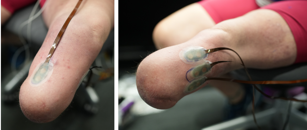
Figure 4-2: Electrode placement for 2-DoF control of the powered ankle-foot prosthesis. Four electrodes are positioned on key muscle groups: Tibialis Anterior (TA), Gastrocnemius (GAS), Tibialis Posterior (TP), and Peroneus Longus (PL).
