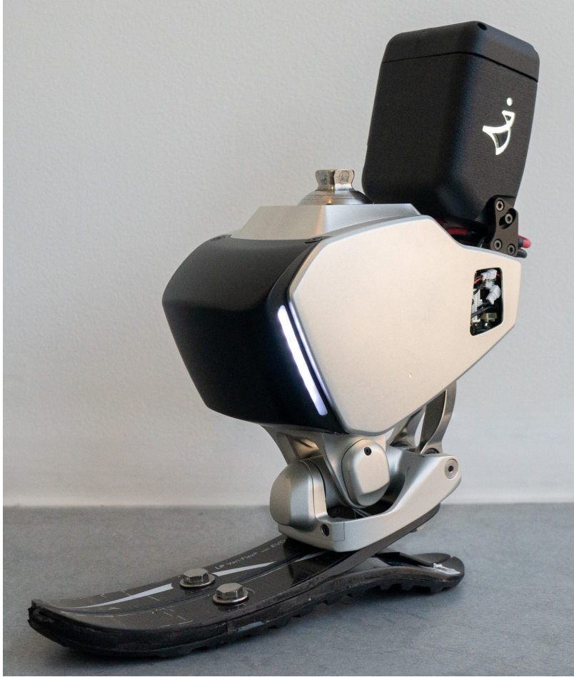
Figure 3-2: Photograph of the physically implemented 2DoF ankle-foot prosthesis prototype.
