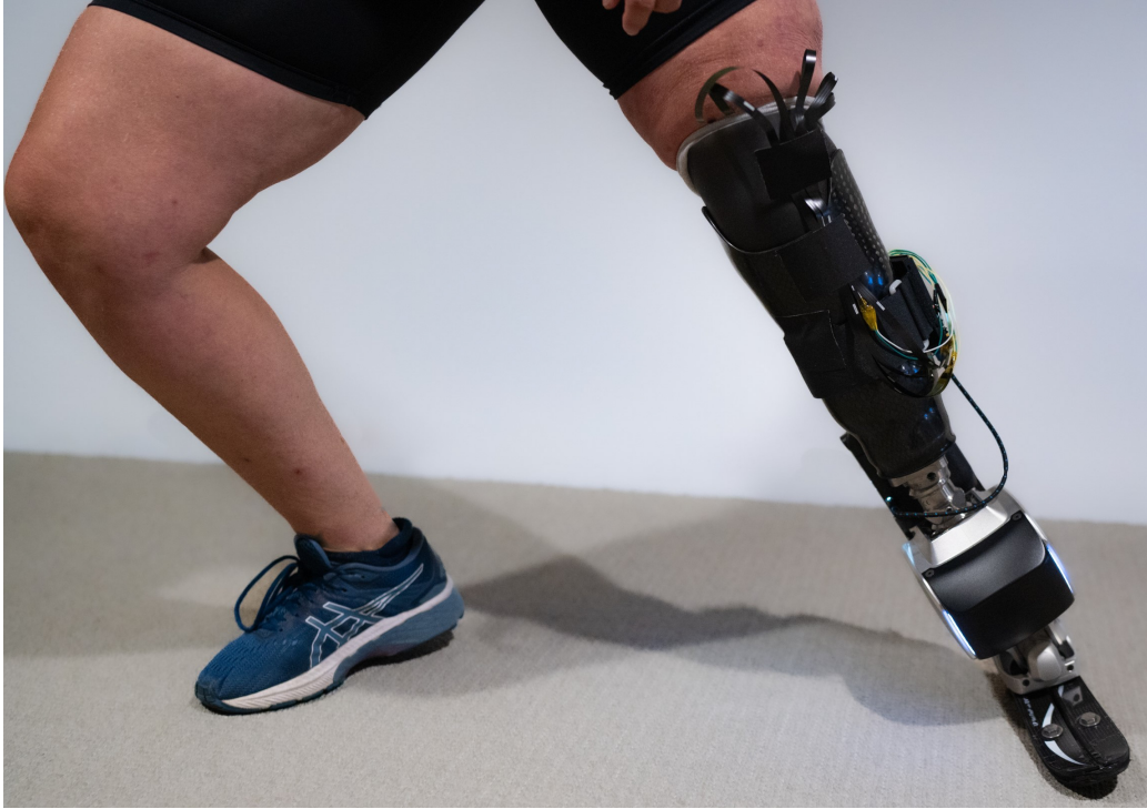
Figure 3-3: Demonstration of a powered prosthetic ankle's range of motion in the frontal plane. This highlights the device's capability to adjust in the frontal plane, allowing for adaptation to uneven terrain and improved stability during various activities.
