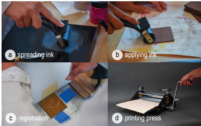
Figure 3: The printmaking procedure comprises (a) coating ink onto the rubber brayer, (b) transferring ink onto the block, (c) registering the block to ensure proper alignment, and (d) using the printing press to transfer ink from the block to the printing surface.
