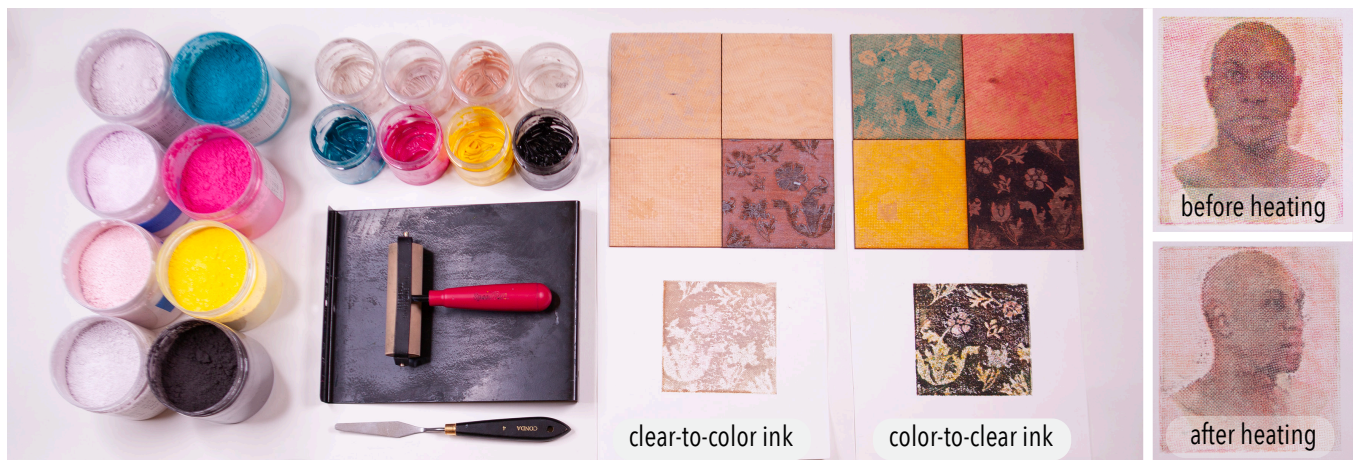
Figure 1: Thermochormorph is a novel workflow for producing visually dynamic relief printed images. Our method combines complementary thermochromic inks with a CMYK-based relief printing process.
