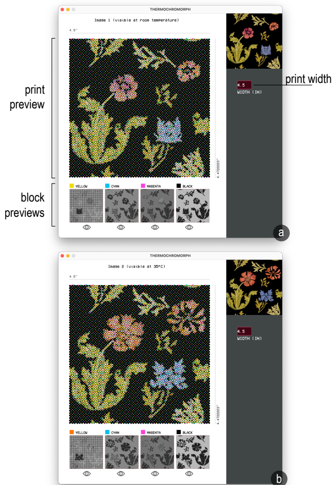
Figure 2: The Thermochromorph interface shows a preview of the CMYK halftone for the target image and provides CMYK block thumbnails below the halftone image. Users can switch between (a) cold and (b) hot image previews.
