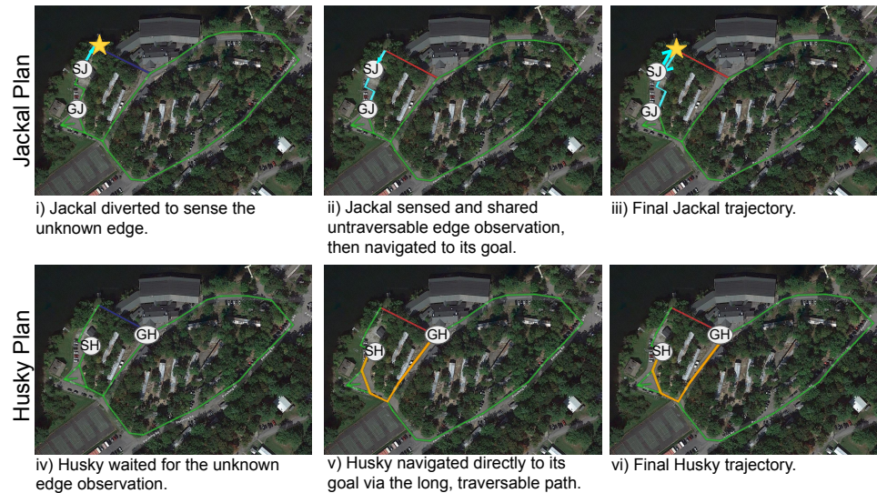
Figure 5.6: Graph-based planning results, Camp Buckner. a) Graph-based plans selected by the non-collaborative baseline planner, visualized over the abstract navigation graph. The Jackal (blue) with start SJ and goal GJ navigated directly to its goal, while the Husky (orange) with start SH and goal GH navigated to the unknown edge, sensed that it was untraversable, and then backtracked to the goal via the long, traversable path. b) Graph-based plans selected by the collaborative planner, visualized over the abstract navigation graph. The Jackal (blue) with start SJ and goal GJ diverted to the gold star to sense the unknown edge, and shared the untraversable edge observation with the Husky. Then, the Jackal navigated to its goal. The Husky (orange) with start SH and goal GH waited to receive the edge observation from the Jackal, then navigated directly to its goal via the long, traversable path. Note that some trajectories were hand-annotated from raw agent outputs for clarity and due to agent/ground station communication drops.
