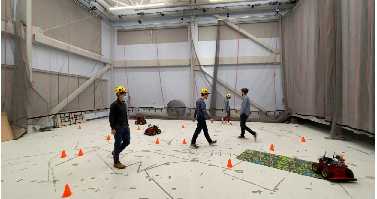
Figure 3.1: MOT hardware experiment in our motion capture room. We use this setup to demonstrate our MOTLEE algorithm’s ability to perform distributed MOT onboard moving robots with localization uncertainty.
