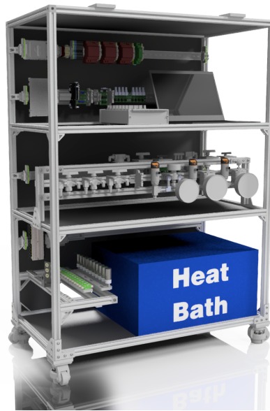
Figure 3.7: We designed the olfactory stimulation control cart to be portable and house all of the components for electronic control, air handling, and fluid handling. 3D rendering of the olfactory stimulation cart design; created prior to assembly and deployment.
