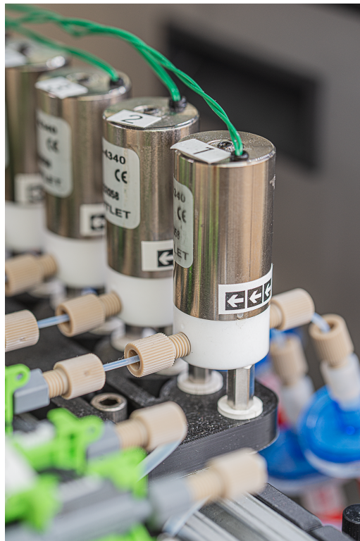
Figure 3.22: We utilized ten solenoid valves to control flow through each of the odor stimulation lines. Photograph solenoids mounted in the stimulation cart for fluid line control.
