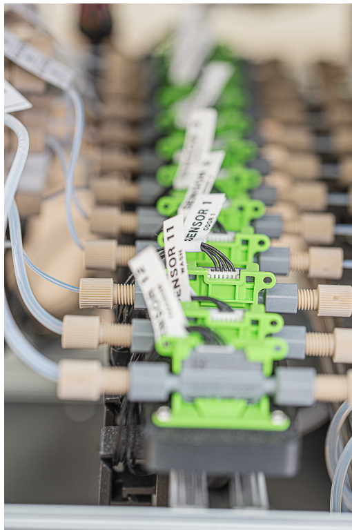
Figure 3.15: We utilized 12 flow sensors to continuously monitor flow through each of the stimulation, wash, and vacuum lines. Photograph of the array of flow sensors on the stimulator cart with electronic and fluidic connections.
