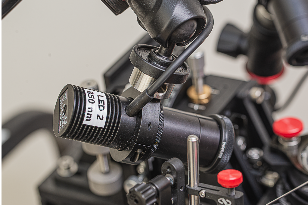
Figure 4.5: Collimated infrared illumination assemblies mounted on positioning arms enable our behavioral camera to capture tail motion.
