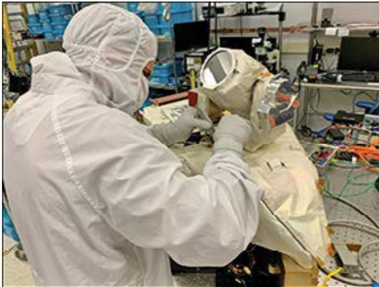
The laboratory is developing two high-rate laser communication terminals for use in space. One terminal, shown here, will be flown on the NASA Artemis II mission, and the other will be deployed on the International Space Station.
