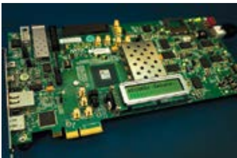
Through dynamic resource monitoring and allocation, this Lincoln Laboratory-developed reconfigurable processor enables very-low-power, secure edge computing for emerging artificial intelligence and machine learning tasks such as voice and image recognition.
