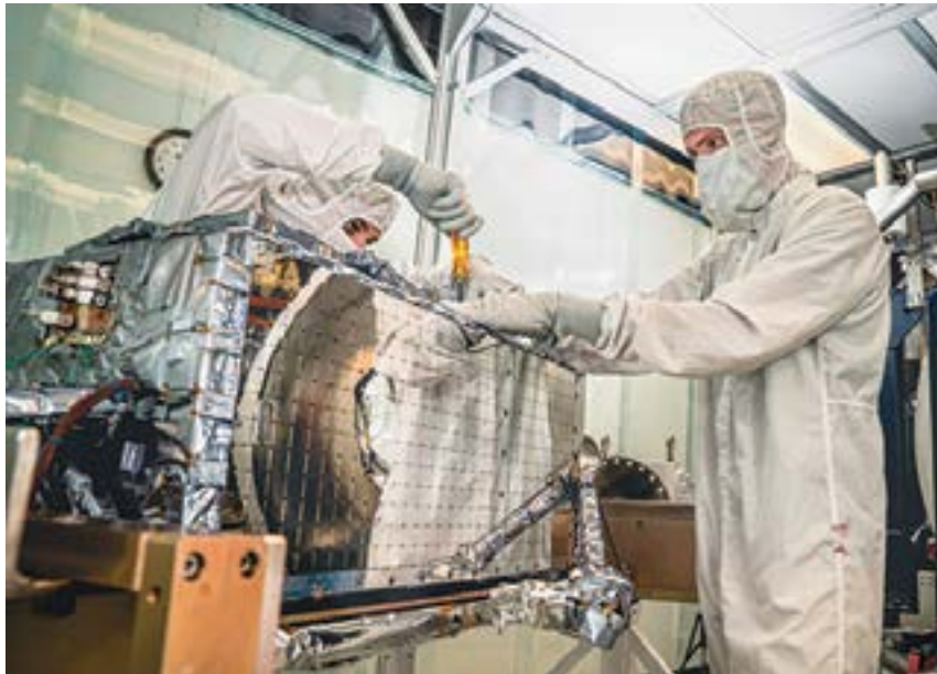
Researchers prepare a situational awareness camera for thermal vacuum testing.
