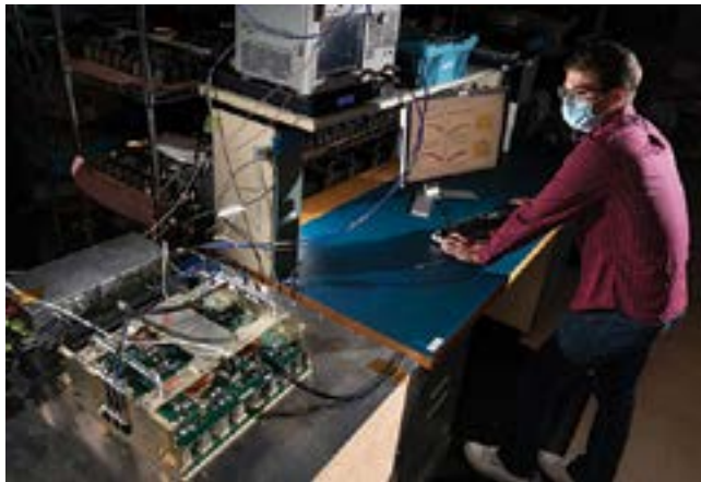
The Dual-Polarization Phased-Array Radar Advanced Technology Demonstrator is a 4-meter array consisting of 76 panels to evaluate improvements in rapid-update weather sensing.
