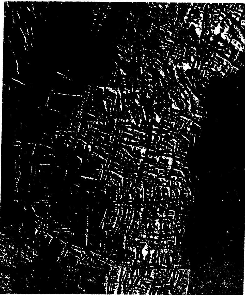
Fig. 47 -- Electron Micrograph of Isotactic Poly(propylene) Crystallized in the Presence of 50% (by weight) Atactic Poly(propylene). Specimen Subsequently Washed in Xylene for 30 Minutes. Magnification 31,000 X.
