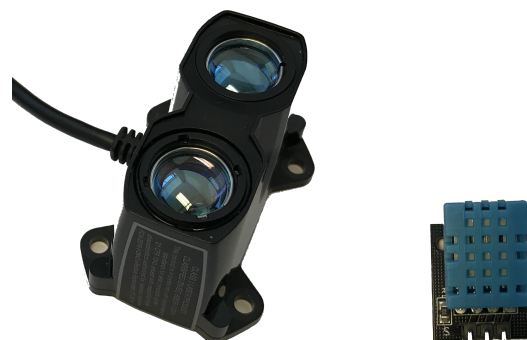
Figure 2: Garmin Lidar Lite r3HP on the left, DHT11 digital temperature and humidity sensor on the right.
