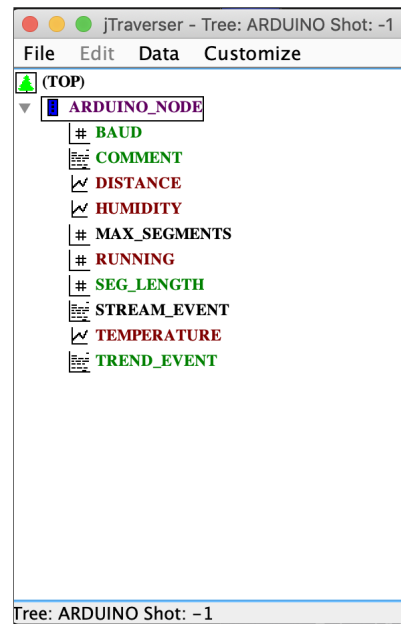
Figure 3: The structure of the MDSplus tree shown by the jTraverser
