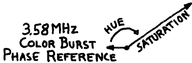
SUBCARRIER PHASOR DIAGRAM SHOWING ENCODING OF THE TWO CHROMINANCE SIGNALS
