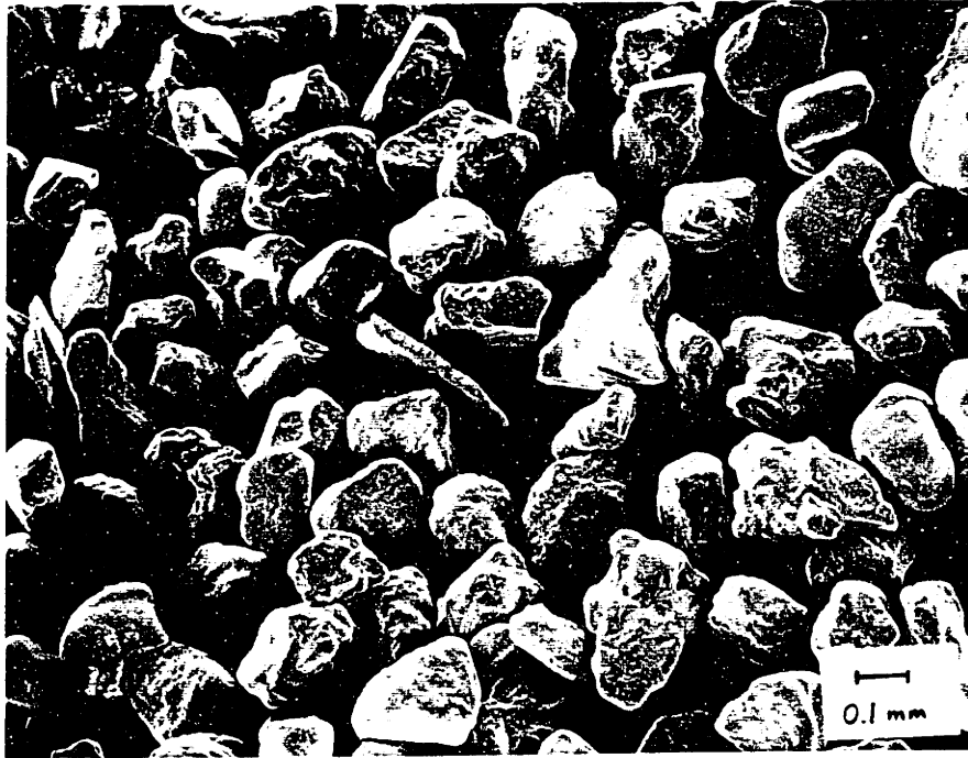
SAND BEFORE TESTING
