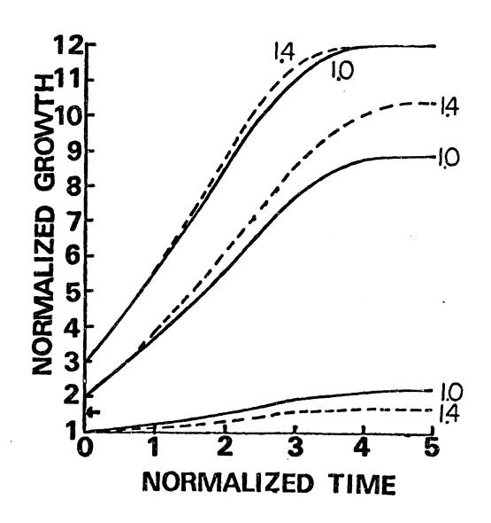
microcarriers having relative diameter 1.4 are shown as broken lines in Figure 1-15. The critical cell number is indicated with an arrow in this Figure. When the inoculum cell concentration is larger than the critical number, the microcarriers of larger diameter show improved cell growth; whereas, at inoculum concentrations lower than the critical number, increasing bead diameter has an adverse effect on cell growth.
