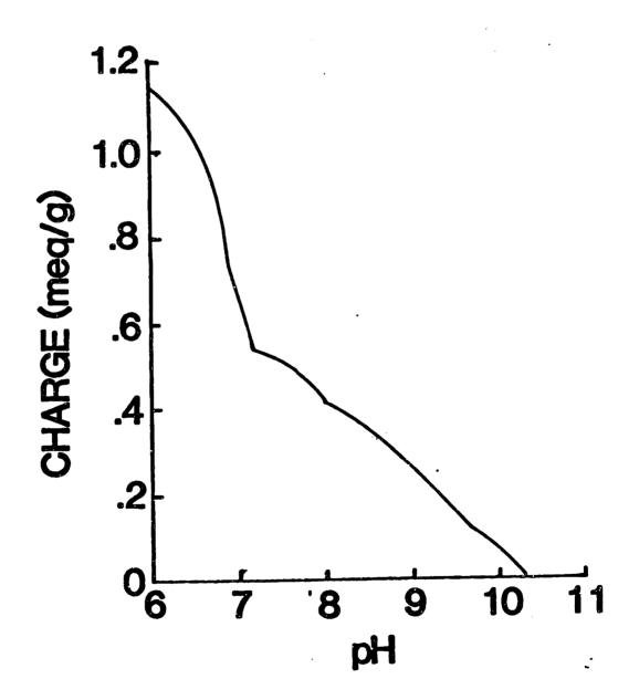
multiple pK<sub>a</sub> values on the titration curve instead of a single reflection point at pH 9.5. This phenomenon has also been reported by the manufacturer of DEAE-Sephadex, Phamarcia Co.(Phamarcia, technical bulletin) and is attributed to side reactions which occur during the coupling of DEAE to Sephadex beads.
