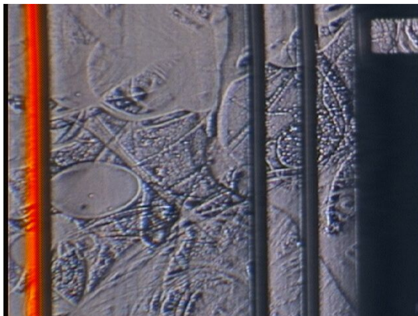
Figure 7-5: Surface roughness after resist burned.
