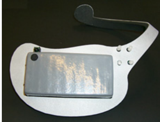
Figure 2-5: Close-up of the sociometer showing the concavity against the body, soft edges and wrap around effect for better wearability
