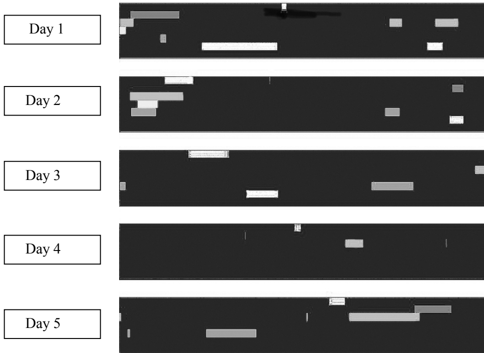
Figure 4-1 - Proximity information for one individual. Each sub-image shows one day's information. Each row within the sub-image corresponds to a different person. Bursty raw sensor data transformed into the contiguous time chunks using HMM.
