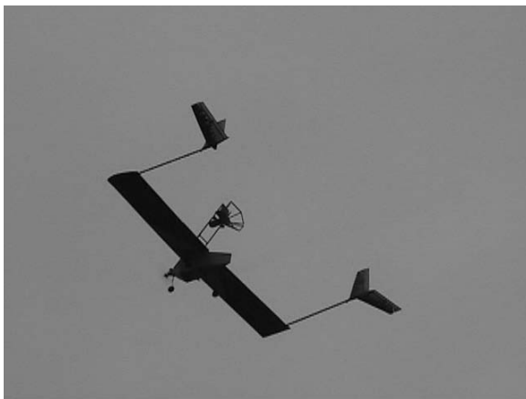
(a) OHS Parent with Truss
