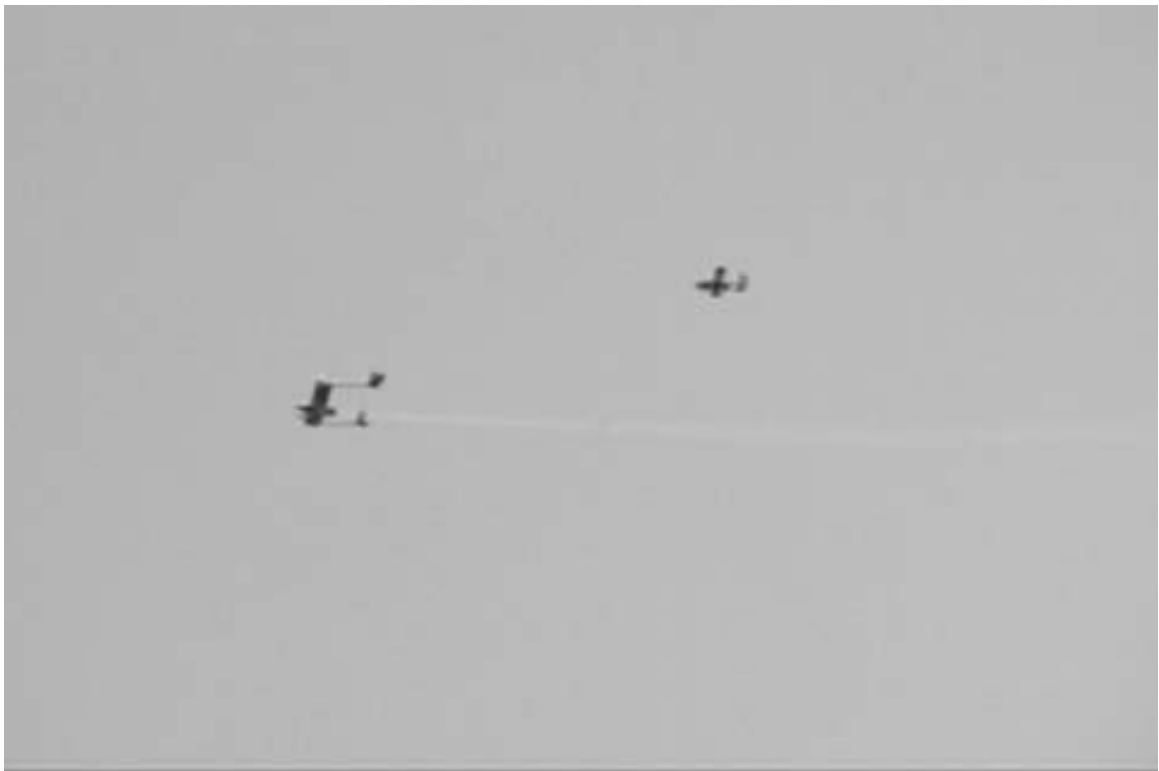
Figure 6-7: Formation Flight during Phase I Flight Test (The Mini is commanded 12 meters behind and 2 meters above the Parent at this moment)
