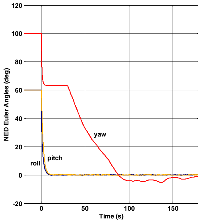
Figure 3-81: Initialization using Gyrocompassing
