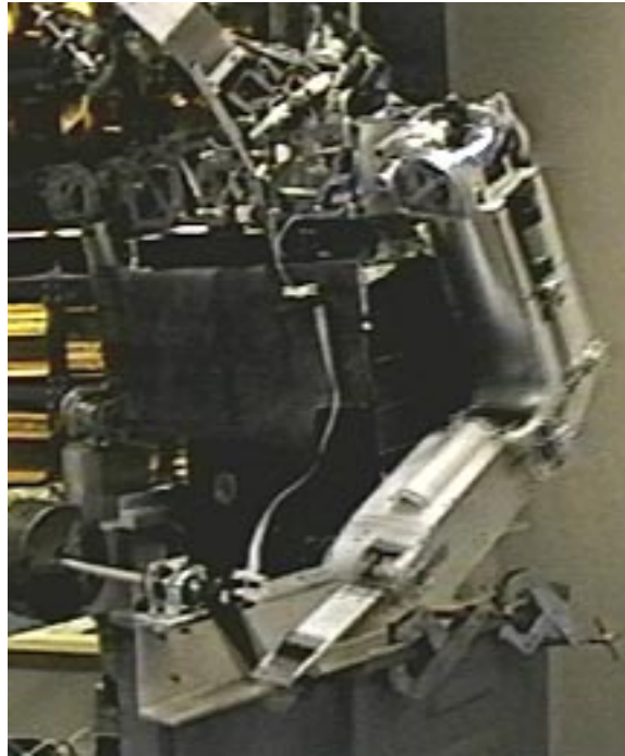
Figure 4-2: REAL Crank turning with one arm. The picture shows the robot using its left arm to turn the crank. Oscillators are used at the shoulder and elbow in this configuration. The oscillators are initially uncoordinated, but use feedback from the motion of the joints to adjust their outputs, so turning the crank.
