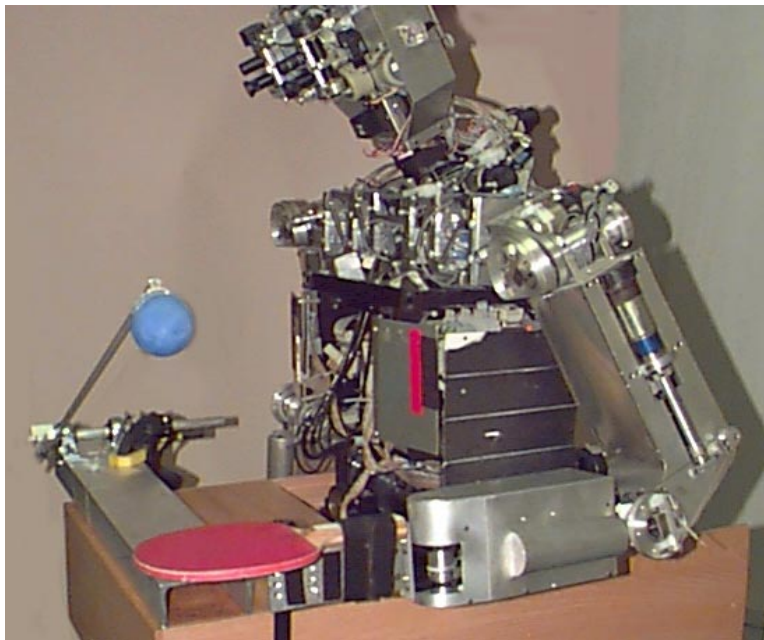
Figure 3-20: Picture of robot in juggling task. The paddle is a table tennis bat attached to the robot's arm. The ball is restrained to travel in one dimension by being mounted on a rotating boom. The angle of the boom is measured using a potentiometer at the pivot point, and this feedback signal is used by the oscillator to coordinate the arm motion with the ball motion.
