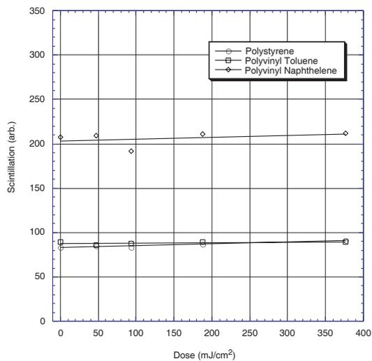
Figure 4-9: Bleaching of base polymers with mercury lamp
