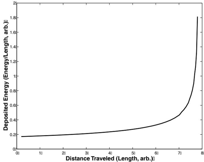
Figure 2-1: Electron energy deposition per unit length versus path length inside a solid material
