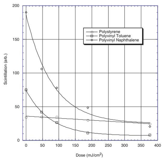
Figure 4-18: Bleaching of polymer bases with 220 nm light
