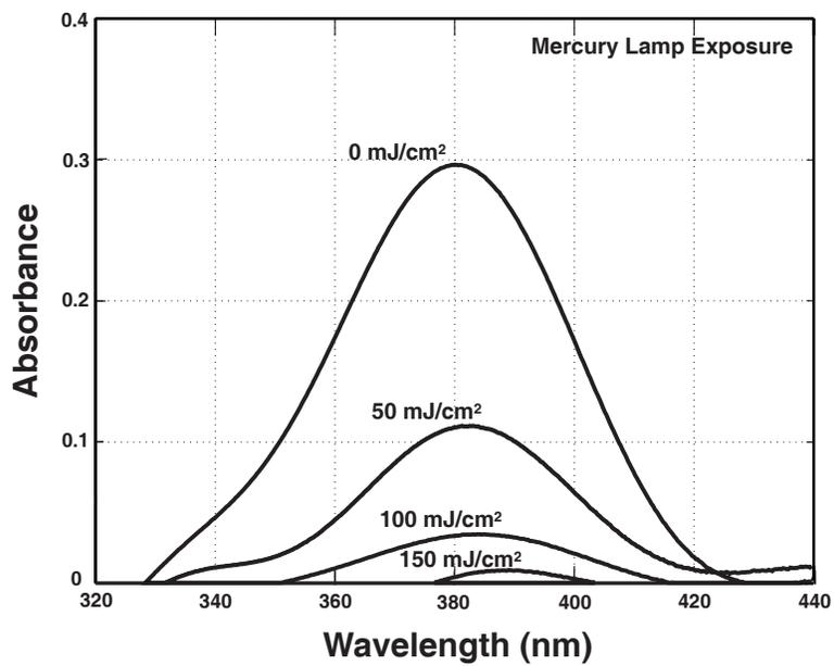
Figure 4-16: Diazonium salt absorbance bands at an arbitrary concentration, showing bleaching with increasing mercury lamp dose
