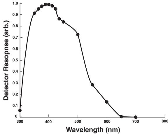
Figure 3-3: Graph of Hamamatsu R6095 photocathode response; after data from Hamamatsu datasheet for photomultiplier tubes R6094,R6095 [21]
