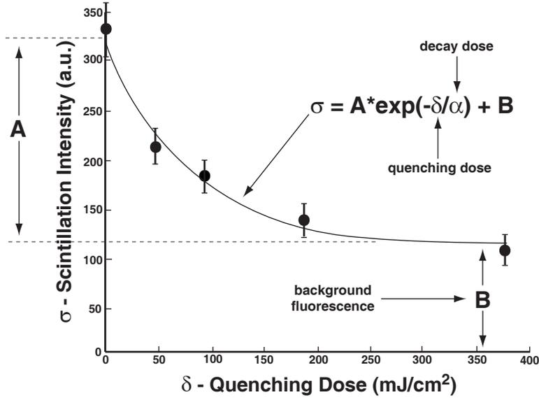
Figure 4-7: Generic bleaching curve with fit equation
