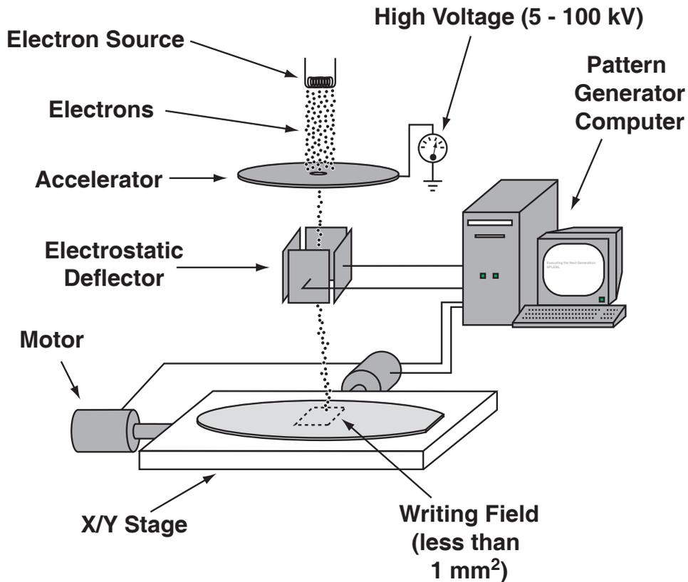
Figure 1-4: Electron-beam lithography
