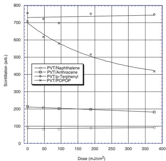
Figure 4-10: Bleaching of scintillating components with mercury lamp
