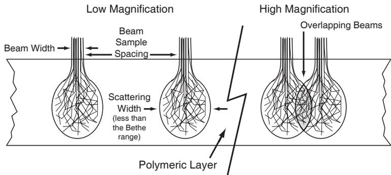
Figure 3-4: SEM mode used to probe for scintillation
