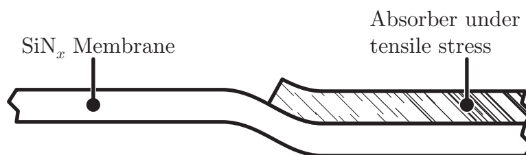
Figure 2-7: Depiction showing an absorber, under tensile stress, causing a membrane to buckle and exhibit OPD.
