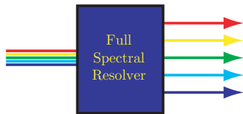
Figure 1-1: Wavelength division multiplexing (WDM) can be used to increase the throughput of simple point-to-point networks. Such systems would use an optical filter device that would fully multiplex and demultiplex the optical signal. A more flexible system would consist of an interconnected WDM network. Such a system would be able route desired signal around the network using an optical filter device that can add and/or drop selected optical wavelengths.
