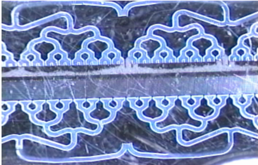
Figure 4-6. Photomicrograph of a reactor loaded with glass beads. Due to momentum effects, the beads load unevenly. However, tapping or shaking leads to the even distribution seen in Figure 4-5.
