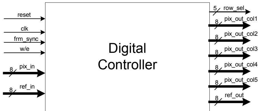
Figure 26. Overall Functional Block Diagram of the Digital Controller
