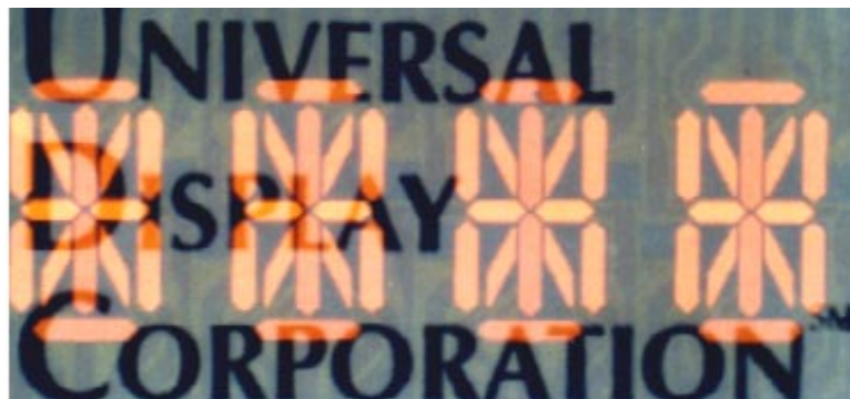
Figure 7. An Alphanumeric Display Made from Transparent OLEDs [2]
