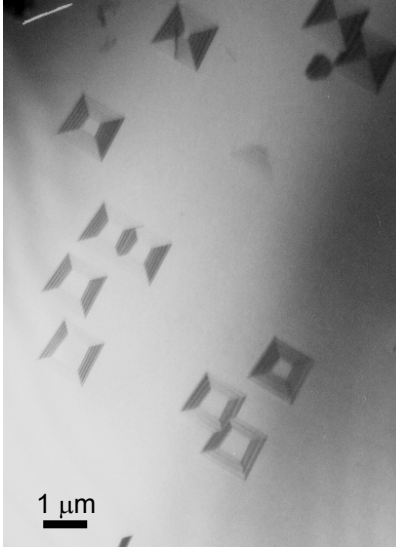
Figure 3.6: Plan-view TEM image of a GaAs film on Ge/GeSi/Si substrate with a high density of pyramidal stacking fault defects. Depending on the orientation of the stacking fault planes with respect to the electron beam they will appear as squares or hourglass shapes in the plan-view microscope image.
