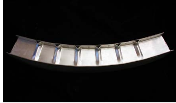
Figure III-18: Segmented construction of planar curves (DCH)
