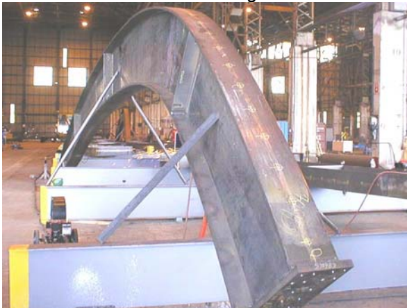
C. Completed rib in shop
