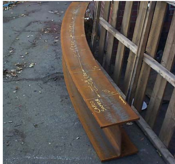
Figure III-19: Arc Segment generated primary structure (MIT)
