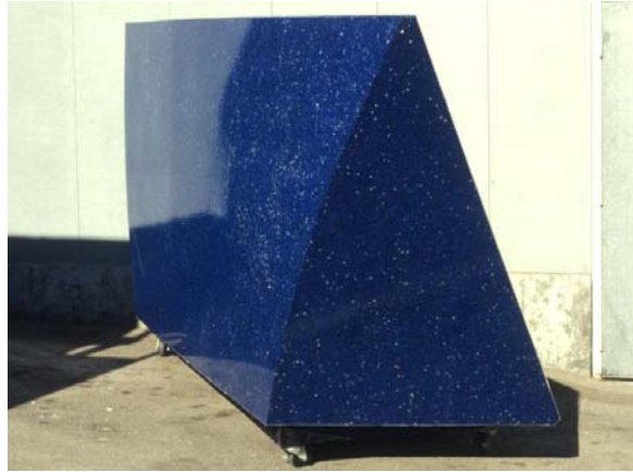
Figure VI-5: Terrazzo mockup (EMP)
