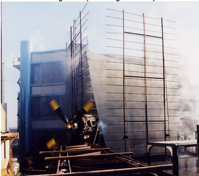
D. Testing under simulated wind and rain conditions
