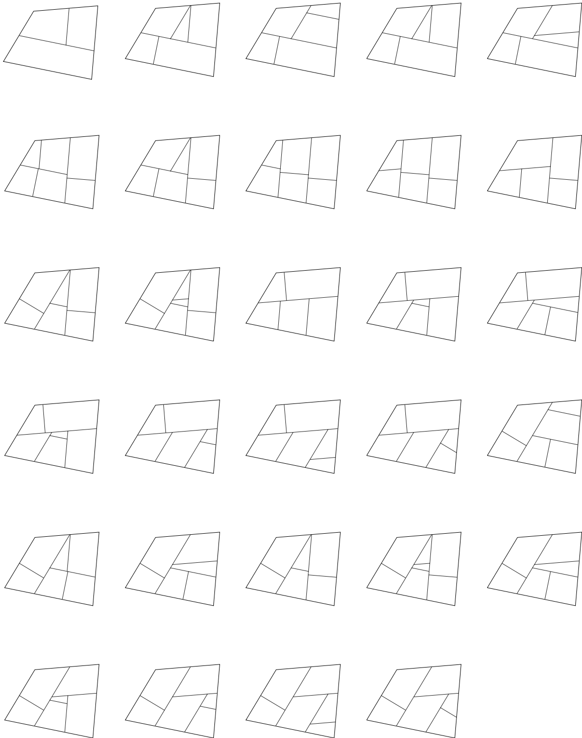
Figure IX-8A Grammar for face sheet layout on panels Test panel sides: 12'7", 10'4", 9', 8'3" 48"x96" material – all 29 permutations
