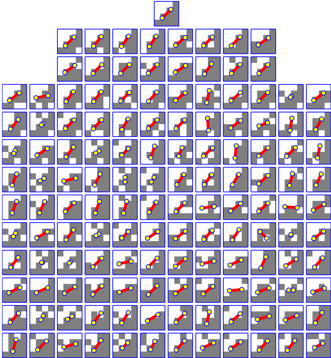
Figure 4-14: Perturbations from an “ideal” view of a diagonal edge. There are now several cases in which little training data is available, and one example of a divergent direction estimate (fourth row from bottom, third column from right).
