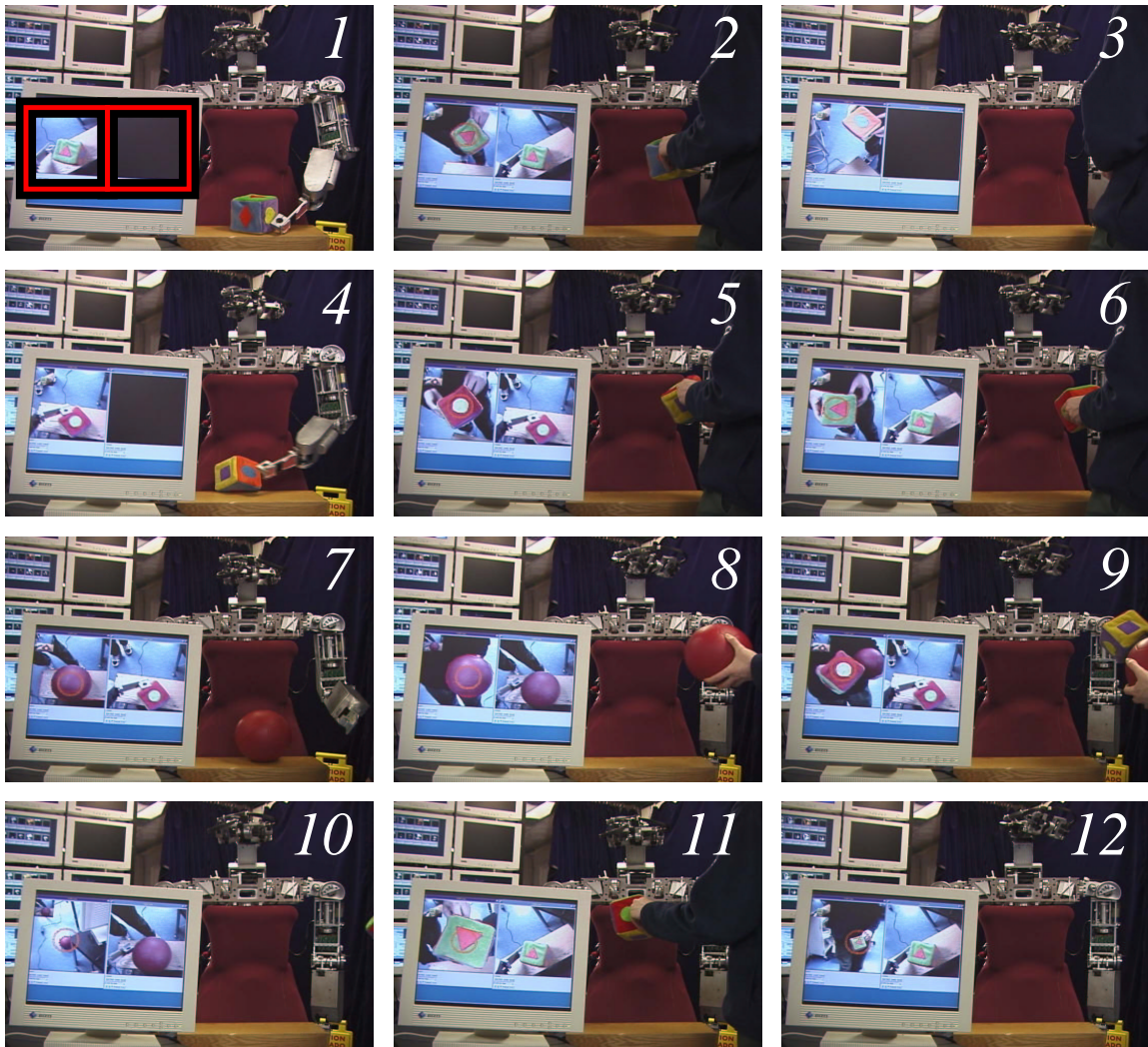
Figure 5-10: This figure shows stills from a three-minute interaction with Cog. The area of the first frame highlighted with a square shows the state of the robot – the left box gives the view from the robot’s camera, the right shows an image it associates with the current view. Initially the robot is not familiar with any objects, so the right box is empty. It is presented with the cube, and pokes it (first frame). Then, if shown the cube again, it recognizes it (this recognition is evidenced by showing an image recorded from when the object was poked). If the cube is turned to another side, the robot no longer recognizes it (third frame). If that side of the cube is presented to the robot to poke (fourth frame), it can then recognize it (fifth frame) and differentiate it from the green side (sixth frame). If it confuses another object with what it has already seen, such as the ball in the seventh frame, this is easily to fix by poking (eighth, ninth frames). The final three frames show the invariance of the recognition system to scale.
