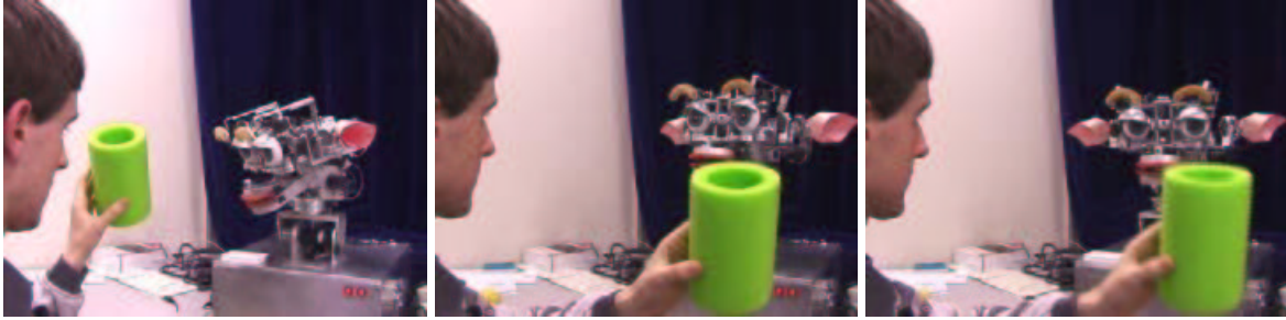
Figure 8-5: These images are from a sequence in which the instructor wanted the robot to attend to the green object as it moved away from a central location. In the first image the robot is clearly attending; in the second it just as clearly has become fixated on the instructors face. Knowing this prompted the instructor to wave the object a little until it regained the robot's attention.
