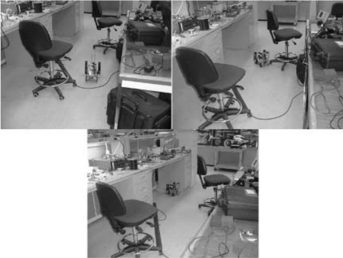
Figure 4-6: The robot avoiding an office chair. The robot approaches a chair (top-left figure) and avoids it by turning left (top-right). The robot continues going forward until encountering the desk drawers, where it avoids it by turning left (bottom). The robot is now caught in a dead end under the desk.
