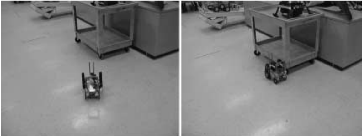
Figure 4-5: The robot avoiding an obstacle in the middle of the lab. The robot approaches the cart from the side, as shown in the left figure, and the robot is able to avoid the obstacle, as shown in the right figure.
