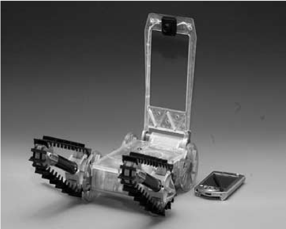
Figure 1-1: Draper Laboratory's High Mobility Tactical Microrobot. The robot is completely controlled by an operator using the IPAQ personal digital assistant (PDA) shown.
