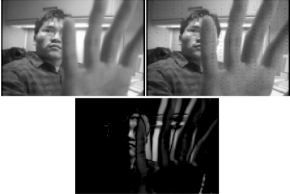
Figure 3-4: Image pair of a scene with motion and their absolute difference image. The top two images show the subject moving his hand between the two frames. The bottom image shows the absolute difference of the image pair, with large magnitudes on the right side where the hand moved. In this case, the image difference imbalance is great enough to mask image noise.
