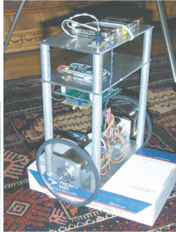
Figure 2-12: “GyroBot” two-wheeled IP platform robot. Created by Larry Barello. The taller version of this robot (at right) is reported to be more stable than the earlier prototype (left). ( http://www.barello.net/Robots/gyrobot/index.htm )
