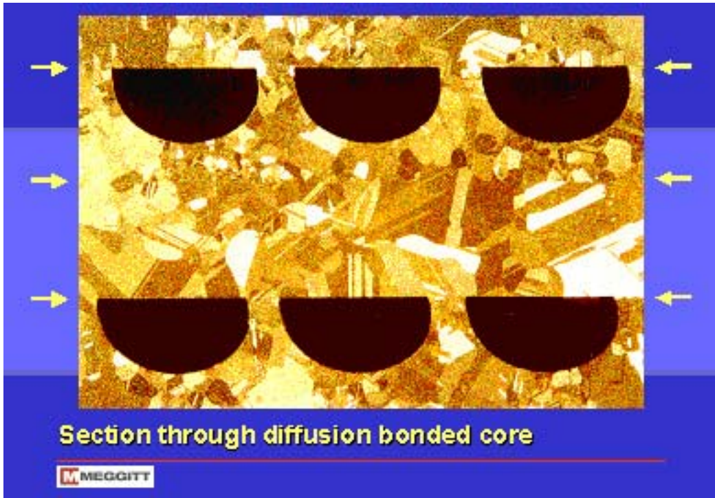
Figure 3.6 Detail of bonded printed circuit plates [7]
