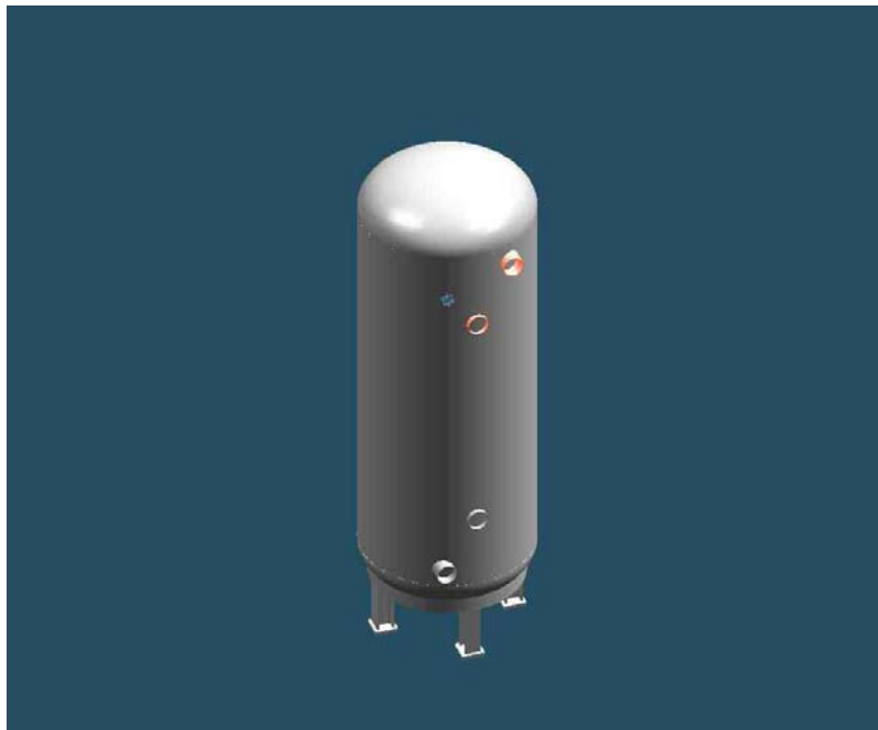
Figure C.1 – IHX unit pressure vessel
