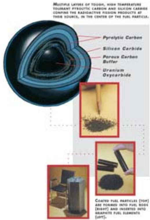
Figure 2.1 Hexagonal fuel element for prismatic core [3]
