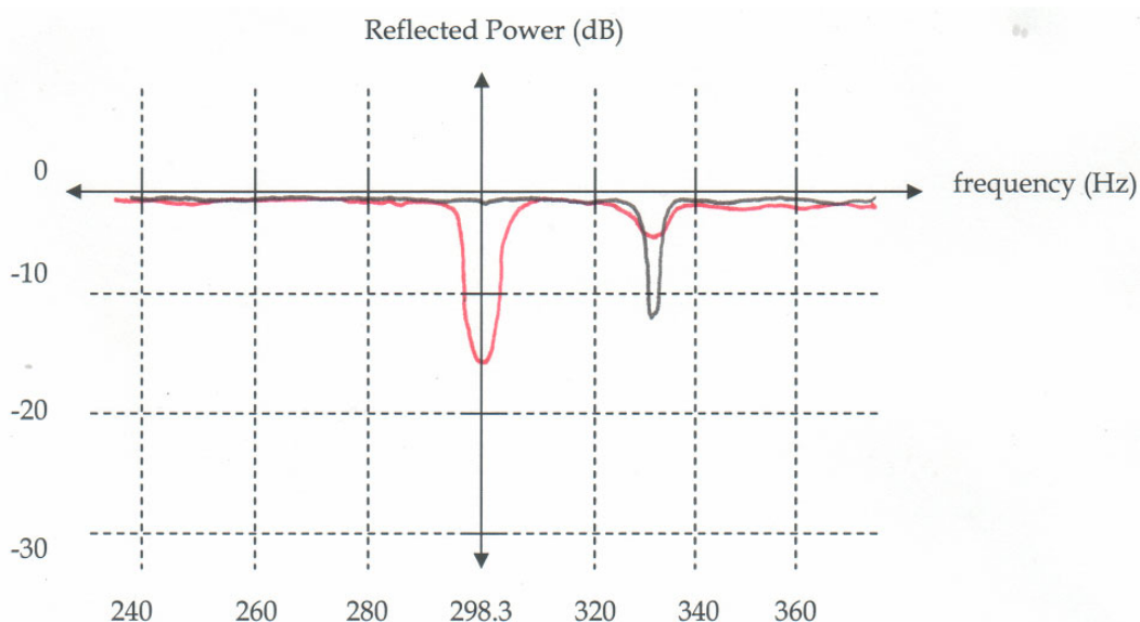
FIGURE 6.5 – REFLECTED POWER RESPONSE FUNCTIONS FOR ONE COIL USED IN HEAD COIL. NOTICE HOW POORLY THE COIL BEHAVES WHEN IT IS UNLOADED SINCE THERE IS NO IMPEDANCE MATCHING (BLACK = UNLOADED; RED = LOADED). SEE APPENDIX (FIGURES A.1 AND A.2) FOR THE TWO OTHER REFLECTED POWER RESPONSE FUNCTIONS.
