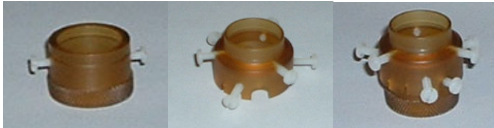
FIGURE 3.3 – (A) HEAD POST FIXTURE A (B) HEAD POST FIXTURE B, AND (C) HEAD POST FIXTURE B MOUNTED ON TOP OF HEAD POST FIXTURE A. HEAD POST FIXTURE A IS SECURED TO THE SKULL WITH DENTAL ACRYLIC AND IS NOT REMOVABLE. THE COOLANT PROBE REMAINS IN HEAD POST FIXTURE B AS TO MAINTAIN A CONSTANT POSITION OVER THE DURATION OF THE STUDY. HEAD POST FIXTURE B IS FIXED TO HEAD POST FIXTURE A DURING THE ACTUAL EXPERIMENT.
