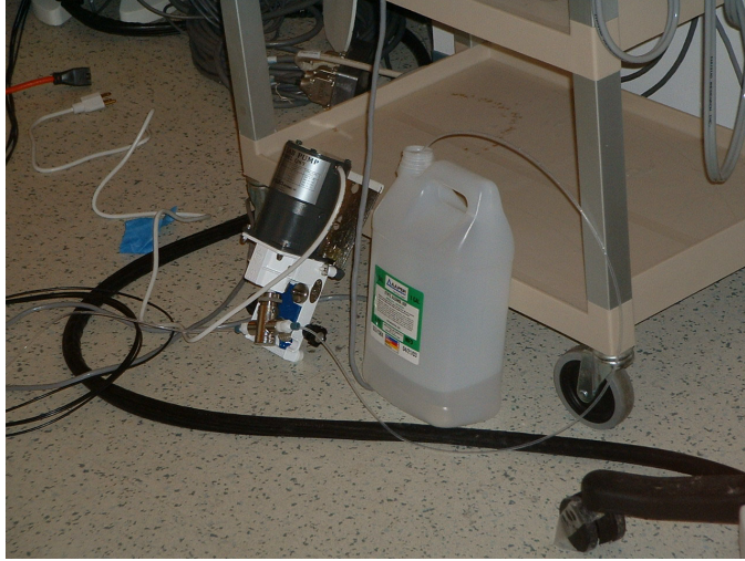
FIGURE A.7 - PUMP AND ETHANOL DUMP (WHERE USED ETHANOL GOES).
