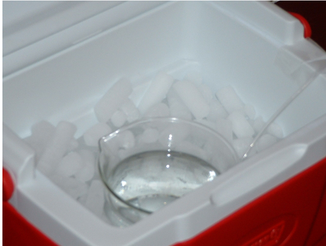
FIGURE A.5 - CONTAINER WITH DRY ICE SURROUND BEAKER OF 100% ETHANOL. THE ETHANOL REACHES TEMPERATURES OF < -50^{\circ}\text{C}
