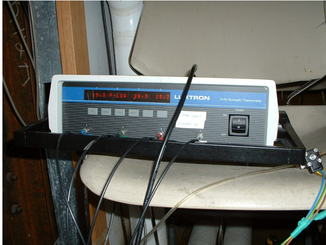
FIGURE A.8 - TEMPERATURE MEASUREMENT DEVICE
