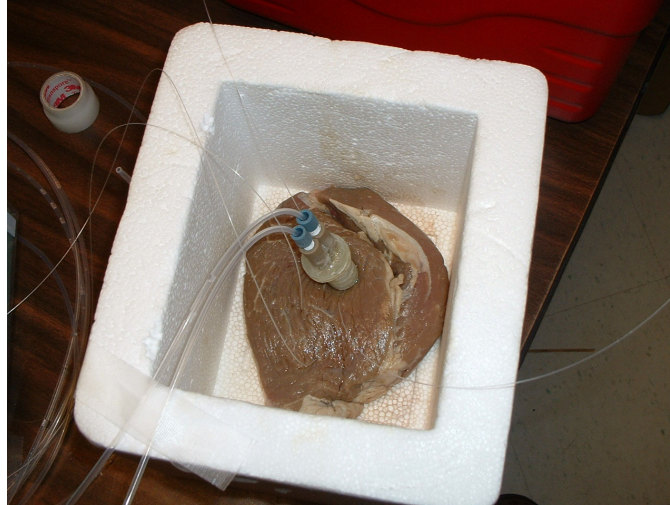
FIGURE A.9 – CLOSE-UP OF ONE TYPE OF THERMOCOUPLE/COOLANT PROBE ARRANGEMENT ON STEAK. THIS SETUP WAS NOT ACTUALLY USED BUT IS SIMILAR IN MOST RESPECTS.
