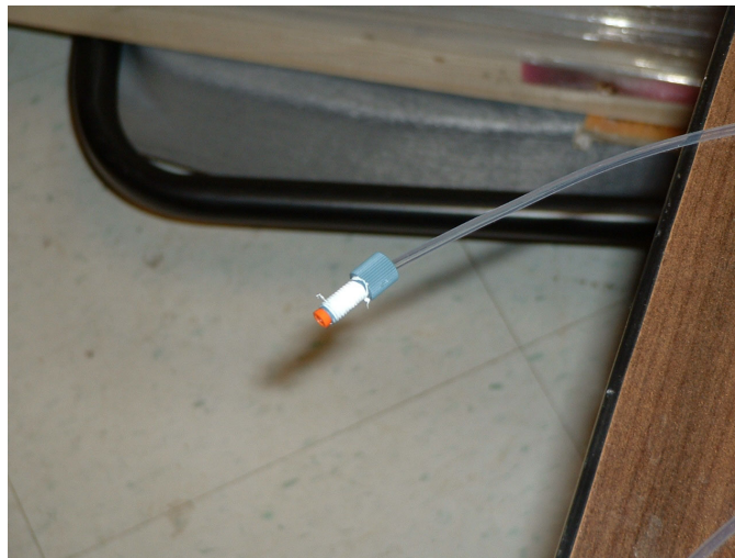
FIGURE A.10 – CLOSE-UP OF FERRULE/NUT COMBINATION USED ON TUBING ENDS TO CONNECT TUBES TO PUMPS AND COOLANT PROBE.
