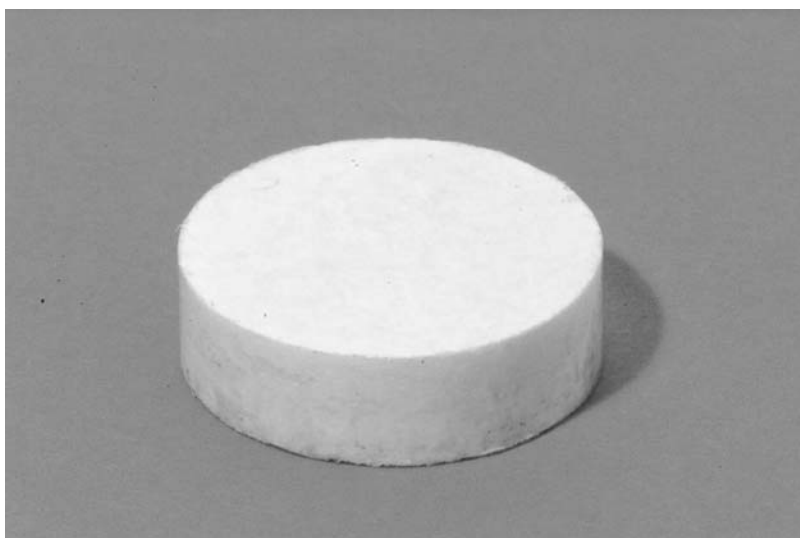
Figure 2.7 Photograph of PLA preform after compression molding of polymer powder in 15/32" cylindrical die at 11,500 psi for one minute and thirty seconds at room temperature. Photo by Richard Holman.
